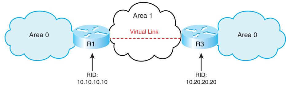
Area 1 is the transit area for the virtual link. Configure each end of a virtual link on the ABRs of the transit area with the command **area area-number virtual-link router-id**. Each end of the link is identified by its RID. The area listed in the command is the transit area, not the area being joined by the link. The configuration for R1 is:
