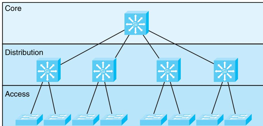
Figure 1-2 is a simple drawing of how the three-layer model might have been built out. A distribution layer-3 switch is used for each building on campus, tying together the access switches on the floors. The core switches link the various buildings together.
