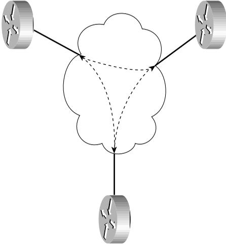
—In a partial mesh, endpoints are connected as needed.
