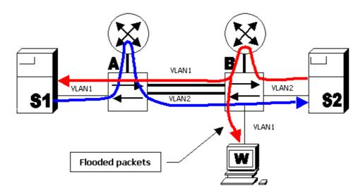
In the diagram above, server S1 in VLAN 1 is running backup (bulk data transfer) to server S2 in VLAN 2. Server S1 has its default gateway pointing to router A's VLAN 1 interface. Server S2 has its default gateway pointing to router B's VLAN 2 interface. Packets from S1 to S2 will follow this path:
