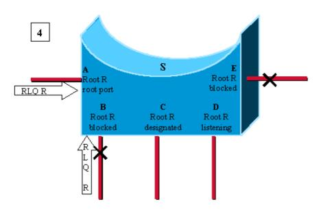
Here, A and B receive a RLQ response confirming R as being the root. As switch S still has connectivity to the root, we can age out immediately the BPDU stored on port E.
