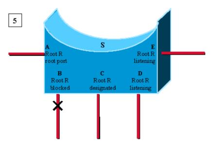
Port E transitions to listering without waiting for max\_age. Usual spanningtree rules then apply to determine whether E and D will eventually go to blocking or forwarding.
