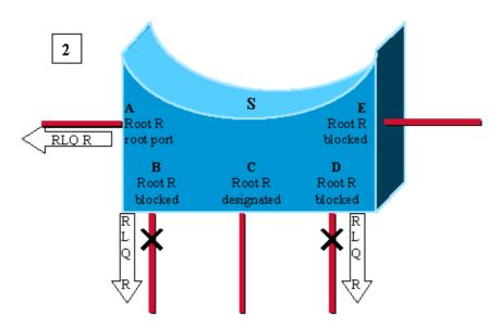
Switch S needs to recheck all its other non-designated ports. It sends out a RLQ request for root R on ports AB and D.
