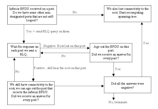
On receipt of an inferior BPDU from a designated bridge, send a RLQ PDU on all non-designated ports except the port where you received the inferior BPDU and self-looped ports. This in order to check that you still hear from the root on ports where you are used to receiving BPDUs. The port where you received the inferior BPDU is excluded because you should already be aware that it suffered from a failure, self-looped and designated ports are not useful, as they don't lead to the root.
