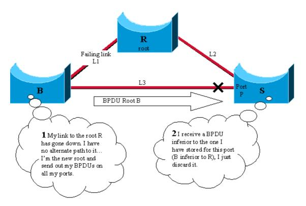
Cisco – Understanding and Configuring Backbone Fast on Catalyst Switches
