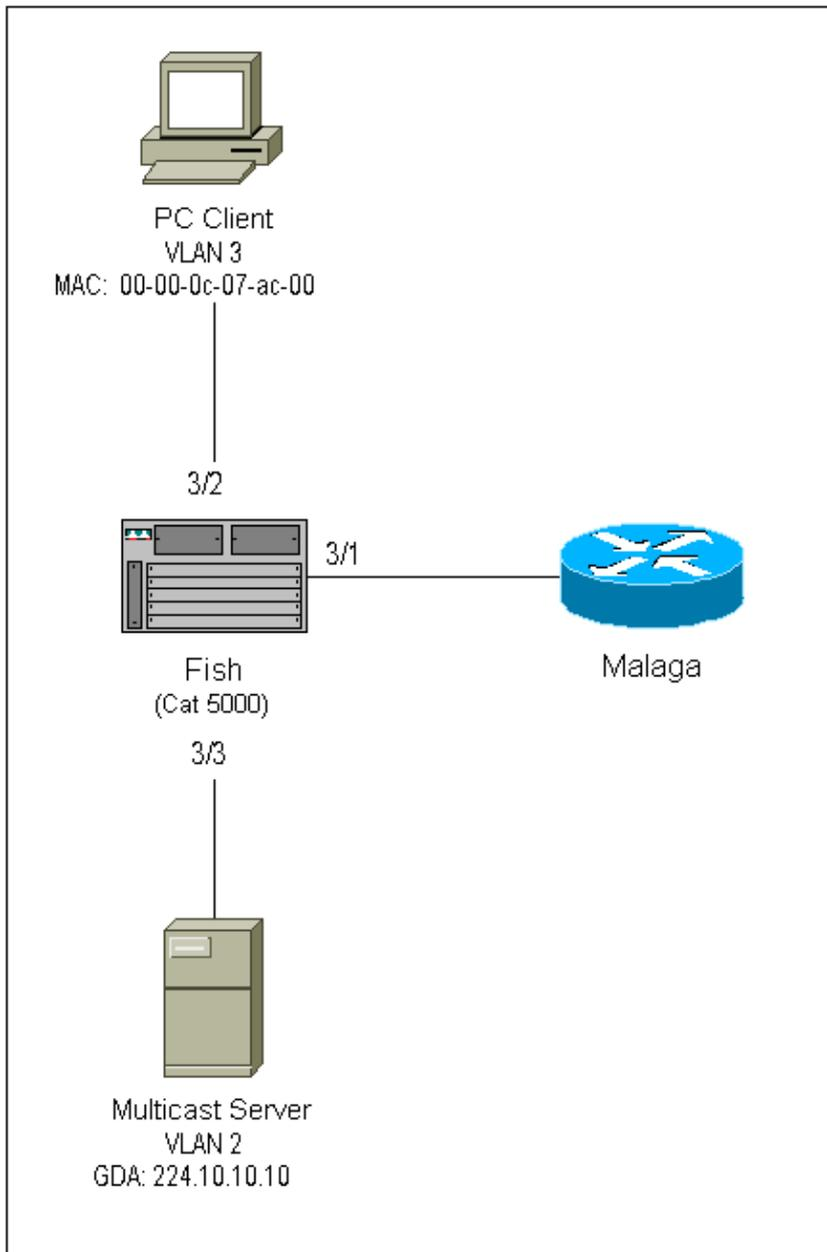
This configuration shows the operations involved as a host joins a group. This configuration also shows the operations as a host leaves a group with Fast-Leave enabled. Sniffer traces and the configuration of the switch and the router are also provided.
