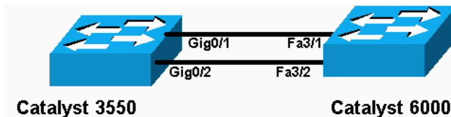
**Note:** The Gigabit Ethernet interface on the Catalyst 3550 is a 10/100/1000 Mbps negotiated Ethernet interface. The Gigabit port on the Catalyst 3550 can also be connected to a FastEthernet (100 Mbps) port on a Catalyst 6500/6000.
