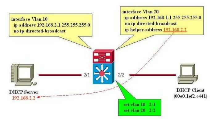
As configured in the diagram above, interface VLAN20 will forward the client's broadcasted DHCPDISCOVER to 192.168.2.2 via interface VLAN10. The DHCP server will fulfill the request via unicast. No further configuration to the router is necessary in this example. The switch ports will need to be configured
