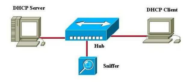
The sniffer trace below is comprised of six frames. These six frames illustrate a working scenario for DHCP, where the DHCP client and server reside on the same physical or logical segment. When troubleshooting DHCP, it is important to match your sniffer trace to the traces below. There may be some differences compared to the traces below, but the general packet flow should be exactly the same. The packet trace follows previous discussions of how DHCP works.
