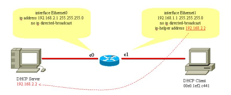
As configured in the diagram above, interface Ethernet1 will forward the client's broadcasted DHCPDISCOVER to 192.168.2.2 via interface Ethernet1. The DHCP server will fulfill the request via unicast. No further configuration to the router is necessary in this example.
