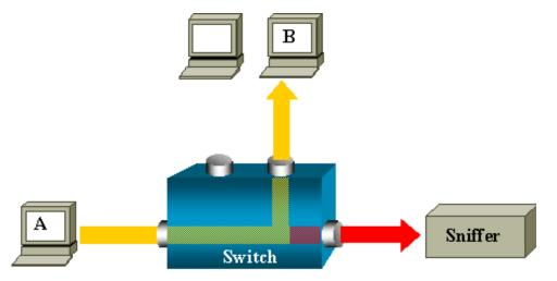
In the above diagram, the sniffer is attached to a port that is configured to receive a copy of every packet that is sent by host A. This port is called a SPAN port. The sections below describe how this feature can be tuned very precisely to do more than just monitor a port.
