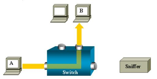
In this configuration, the sniffer only captures traffic flooded to all ports, such as broadcast traffic, multicast traffic with CGMP or Internet Group Management Protocol (IGMP) snooping disabled, and unknown unicast traffic. Unicast flooding happens when the switch does not have the destination MAC in its content-addressable memory (CAM) table. It does not know where to send the traffic, and it floods the packets to all the ports in the destination VLAN.
