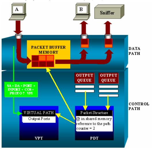
On a Catalyst 4500/4000, you can distinguish the data path, which corresponds to the real transfer of data within the switch, from the control path, where all the decisions are taken.
