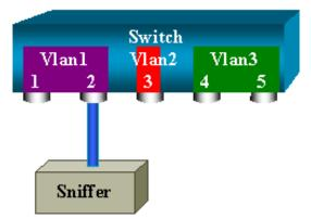
This diagram represents part of a single line card located in slot 6 of a Catalyst 6500/6000 switch. Ports 6/1 and 6/2 belong to VLAN 1, port 6/3 belongs to VLAN 2, and ports 6/4 and 6/5 belong to VLAN 3. Connect a sniffer to port 6/2 and use it as a monitor port in several different cases.
