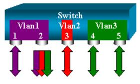
The **set span** *source\_ports destination\_port* command allows the user to specify more than one source port. Simply list all the ports on which you want to implement the SPAN, separated by commas. The command line interpreter also allows you to specify a range of ports by using the hyphen. The example below illustrates this ability; SPAN on port 6/1 and a range of three ports starting from 6/3 are used. There can only be one destination port, and it is always specified after the SPAN source.
