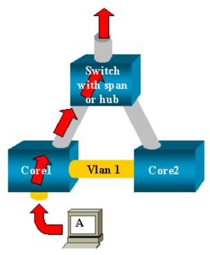
Each of two core switches, linked by a trunk, for instance, has several servers, clients or other bridges connected to them. The administrator wants to monitor VLAN 1, which is appearing on several bridges with SPAN. To achieve that, he creates a SPAN session monitoring the whole VLAN 1 on each core switch, and, to merge these two sessions, connects the destination port to the same hub (or the same switch, using another SPAN session).
