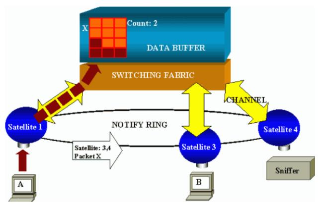
The ports of the switch are attached to satellites that communicate to a switching fabric via radial channels. On the top of that, all the satellites are interconnected via a high-speed notify ring, dedicated to signaling traffic.
