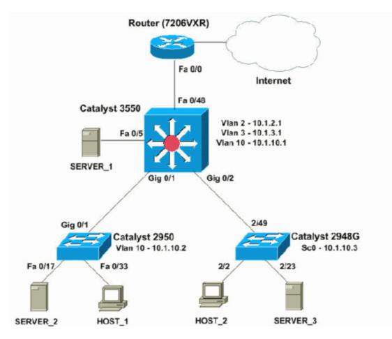
In this diagram, a small sample network with the Catalyst 3550 provides interVLAN routing between the various segments. By default, the Catalyst 3550 switch acts as an L2 device with disablement of IP routing. In order to make the switch function as an L3 device and provide interVLAN routing, you must enable IP routing globally.
