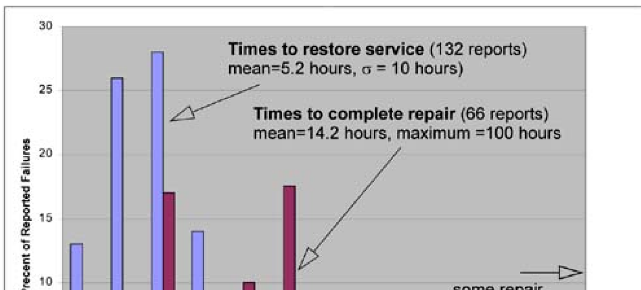
Figure 3-2. Histogram of service restoration and cable repair times (data from [Craw93]).
