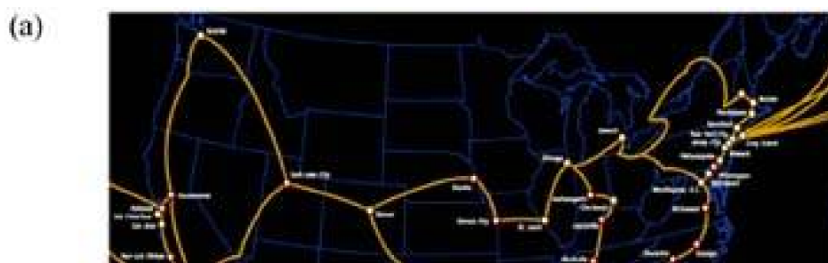
Figure 1-14. The range of fiber network topologies: (a) a sparse North American long-haul route-structure ( \bar{d} \approx 2.2 ), (b) a more richly connected European fiber backbone route structure ( \bar{d} \approx 4.4 ), (c) another European regional network ( \bar{d} \approx 4.1 ).
