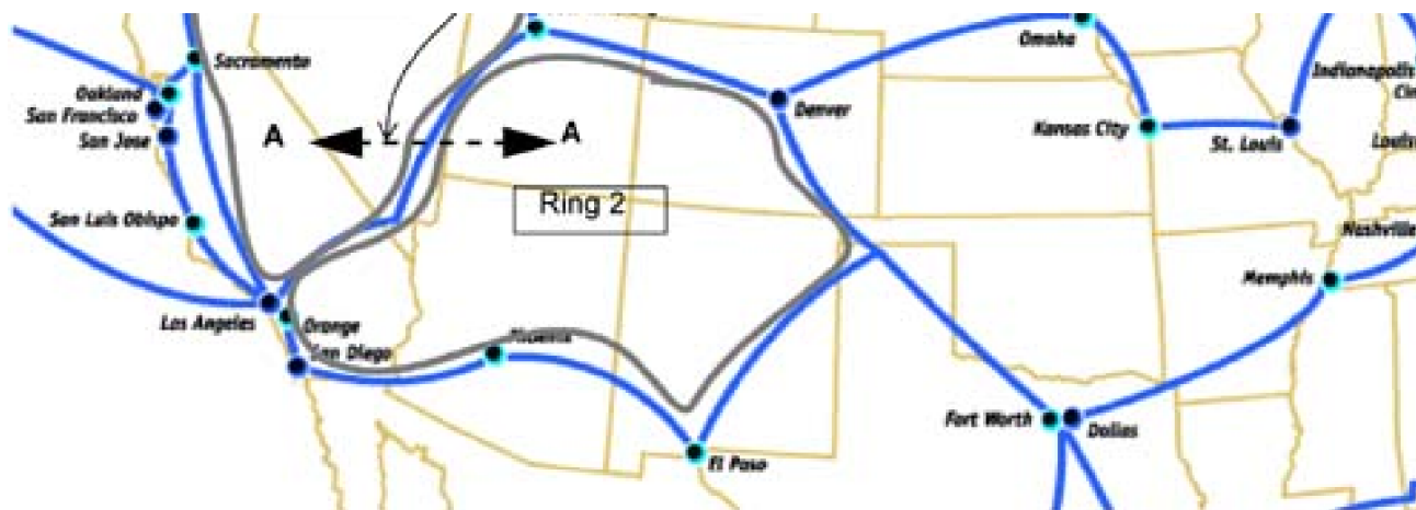
Figure 10-6. Cross-section view with enhanced rings—redundancy of 275% at 40% working fill by coordinating access to a common protection span.
