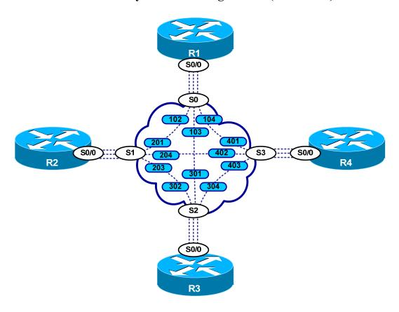
Provided below is the Frame-Relay switch configuration. If you enter this configuration into a router acting as a Frame-Switch and you cable up your pod in the manner displayed on this page, you will have configured a full-mesh Frame-Relay topology.
