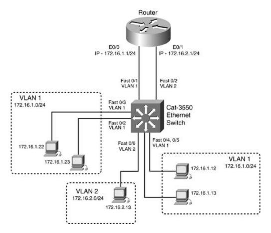
Figure 1-2. Per-Interface VLAN routing
