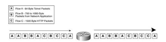
Figure 6-1. Example of FIFO Queuing
