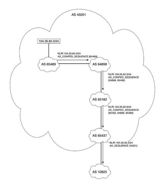
Figure 7-42 illustrates the various parts of a configuration and the roles that routers play, both inside and outside the confederation.
