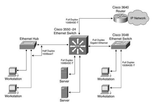
Figure 1-11. Ethernet Network Duplex Settings
