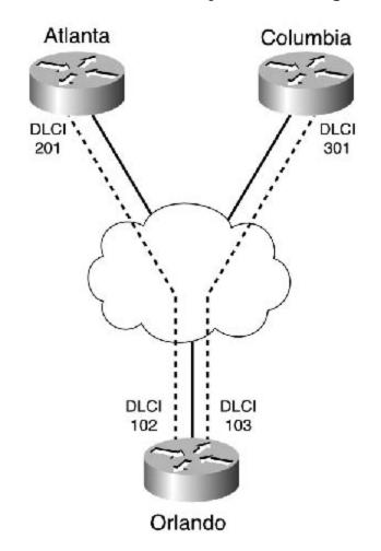
Figure 6-13. Frame Relay DLCI Configuration
