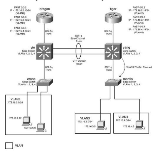
Figure 1-17. VLAN Trunking and STP
