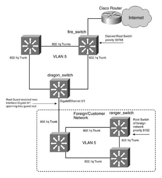
Figure 1-25. Root Guard Placement
