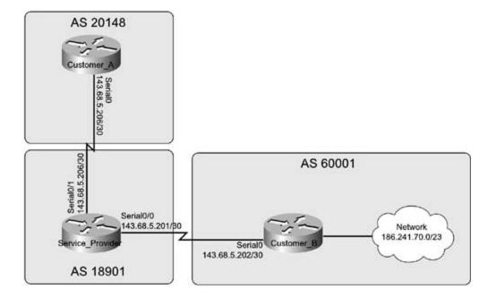
Figure 9-19. Service Provider to Customer Network
