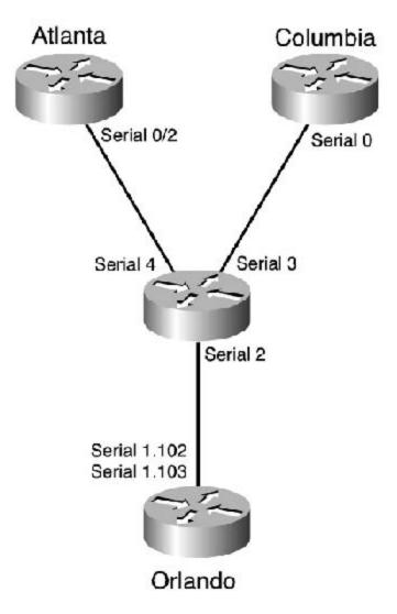
• Configure the Frame Relay as shown in Figure 6-13 using the IP addressing and DLCI assignments shown in Table 6-24.
