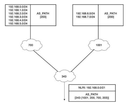
Figure 7-25. AS\_PATH Attribute with an AS\_SET
