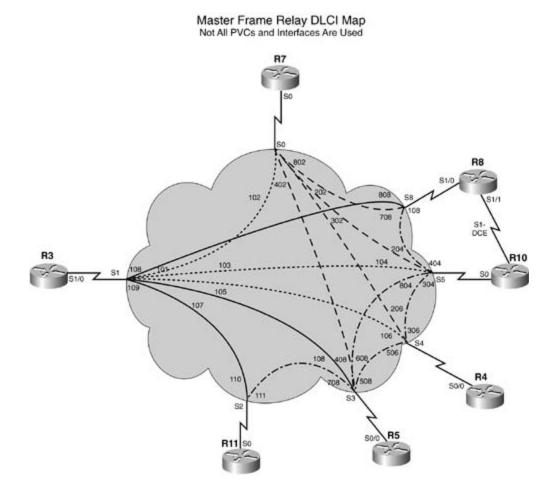
Figure 10-9. Frame Relay Switch Configuration
