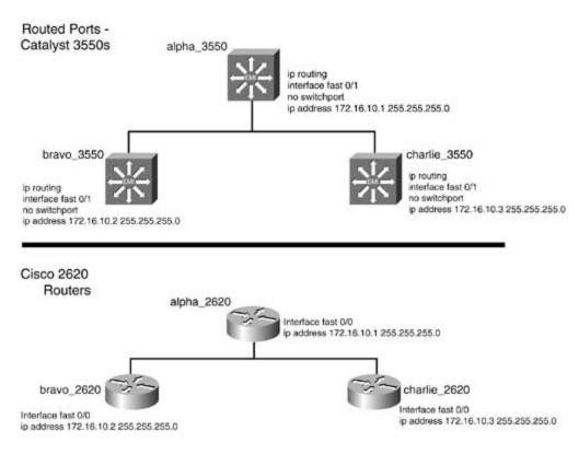
Figure 1-22. Routed Port Comparison
