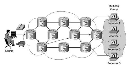
Figure 3-1. Object of Multicast: One-to-Many Routing
