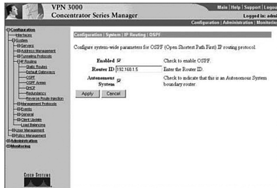
Figure 9-3 Configuration | System | IP Routing | OSPF
