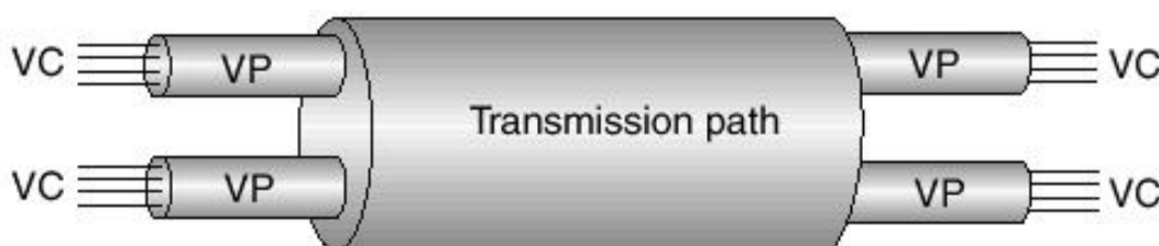
Figure 2-12. ATM Virtual Circuits from a Customer Perspective
