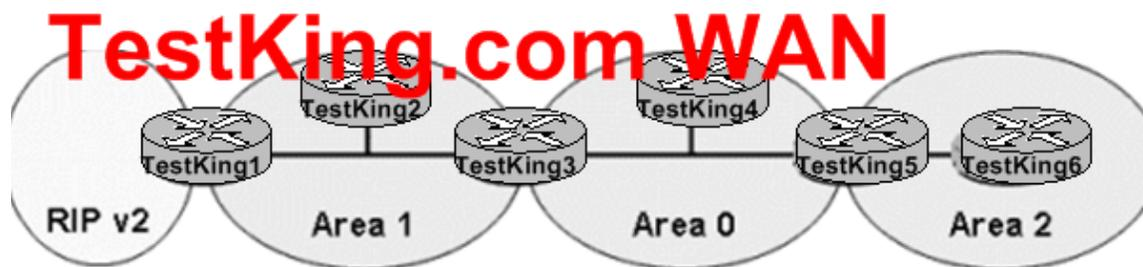
Area 1 is an OSPF Not So Stubby Area (NSSA). What type of LSA will TestKing3 send out area 0 to indicate the presence of an ASBR in Area 1?
