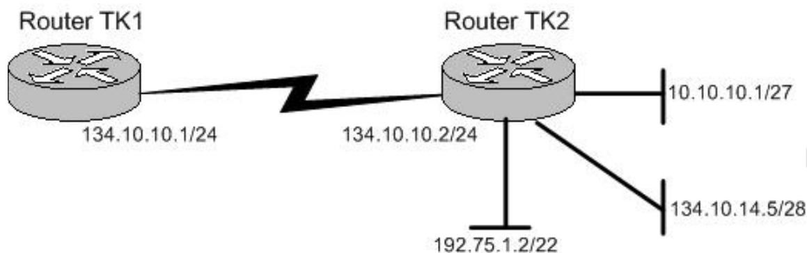
Both Router TK1 and Router TK2 are running RIPv1. Both routers are configured to advertise all of their attached networks via RIP. Which of the networks connected to Router TK2 will be advertised to Router TK1?
