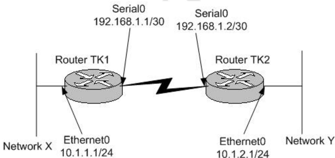
You wish to set up an IPSec VPN between routers TK1 and TK2. Now, which of the following crypto access-lists must be configured on Router TK1 in order to send LAN to LAN traffic across the encrypted VPN tunnel?
