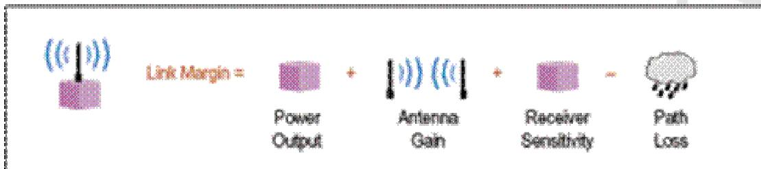
The overall link margin of a system includes transmission power output, antenna gain, receiver sensitivity and path loss. Path loss is caused by cable and antenna attenuation, air content and obstacles preventing line-of-sight conditions.
