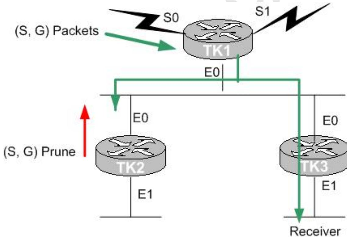
Router TK2 sends a (S, G) Prune message to the LAN segment. Will this cause router TK1 to stop the multicast flow to router TK3?
