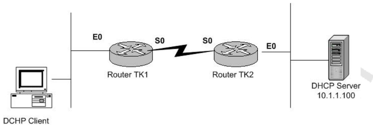
You want all PC's at TK1 to be able to obtain their IP address dynamically from the DHCP server that resides at TK2. Currently, the hosts are not able to obtain an IP address, and they are receiving error messages saying that the DHCP server is busy or is unavailable. What must be done to enable these PC's to obtain dynamic IP addresses.
