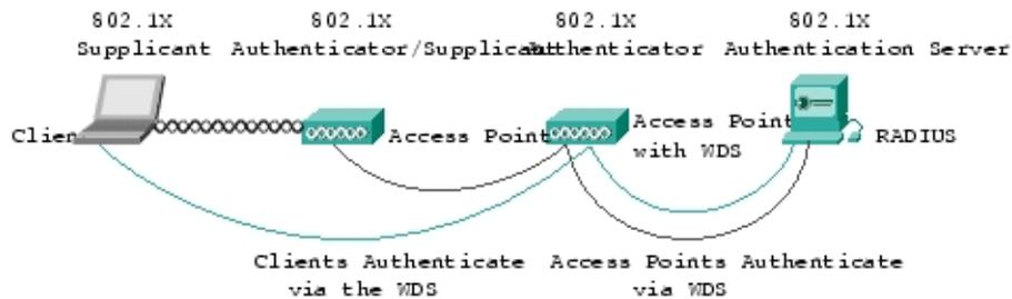
The WDS function is written in Cisco IOS Software and initially runs on Cisco IOS Software on Cisco Aironet access points only. In the future, WDS be available in Cisco router and switch infrastructure products.
