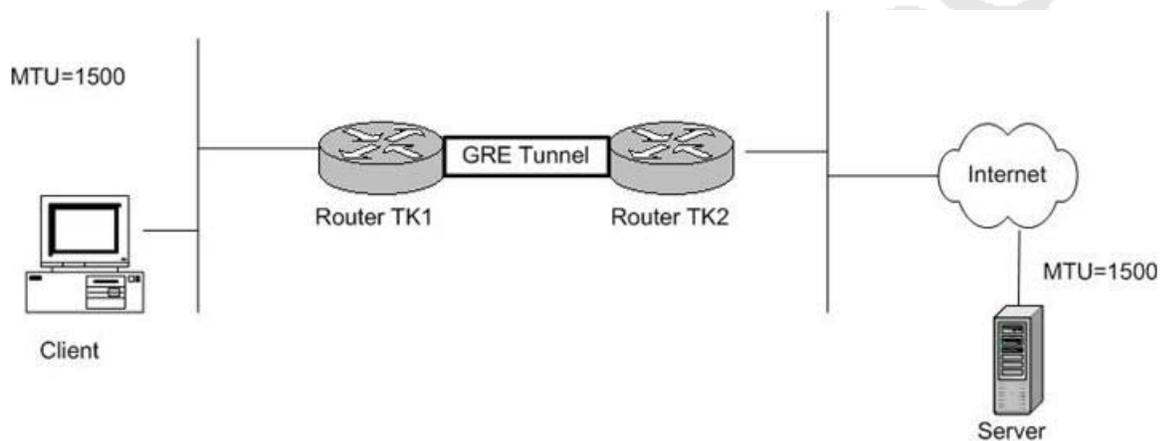
There is a GRE tunnel between two routers, TK1 and TK2. Small files can be sent and received through this tunnel, but large files can not. In addition to this, many web pages are not able to be seen.
