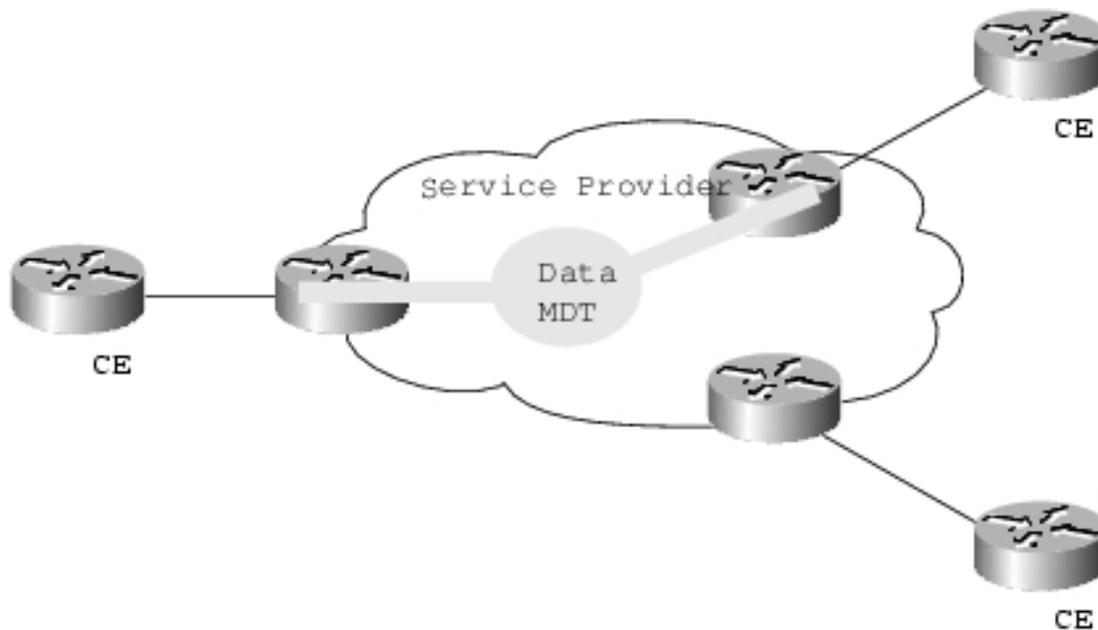
This diagram indicates that the Data MDT is only joined by those PE routers that have CE routers who are intended recipients of the data. PE routers signal use of Data-MDT via a UDP packet on port number 3232, which is sent via the default MDT. This packet contains an all-PIM routers message, indicating the group to be joined if required.
