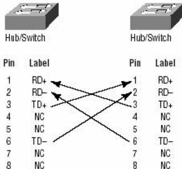
Notice that pin 1 on one side connects to pin 3 on the other side, and pin 2 connects to pin 6 on the opposite end.
