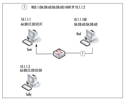
Figure 7.5 ARP Spoofing (Cache Poisoning)
