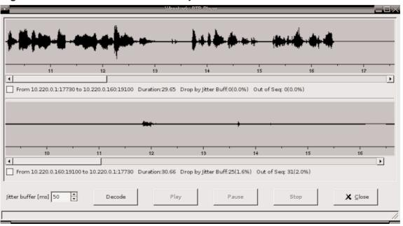
Figure 5.7 Decoded Wireshark RTP Player
