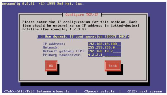
netconfig will prompt you for the IP address, netmask, gateway, and nameserver of your network. Enter these as appropriate for the system. After confirming these settings, the utility will exit. Reboot the system, and the new network settings will take effect.
