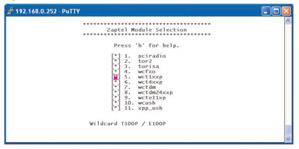
Menuselect lists a description at the bottom of the screen that explains which module supports which card. You can safely deselect any cards your system does not have installed. If a dependency is broken, menuselect will inform you of this and allow you to correct the configuration.
