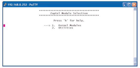
You can navigate through menuselect with the arrow keys—up and down scroll through the menu, left exits to the previous menu. Pressing **Enter** or the **Spacebar** will select/deselect a module or enter a menu. **F8** will select all the modules, and **F7** will deselect all the modules. To save and quit, press **x**, and to quit without saving, press **q**. If you forget any of the keys, press **h** and the help screen will be displayed, as shown in Figure 2.20.
