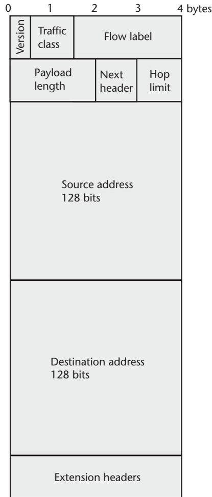
Figure 1.9 IPv6 header.
