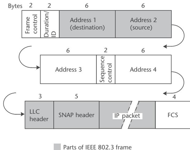
Figure 7.16 IEEE 802.11 frame incorporating IEEE 802.3 frame.
