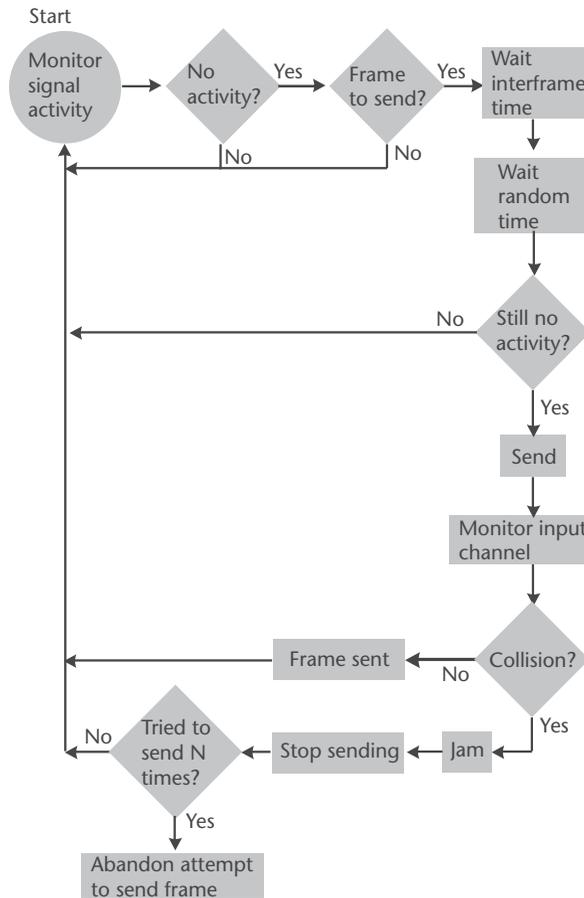
**Figure 3.2** Principle of carrier sense multiple access with collision detection.
