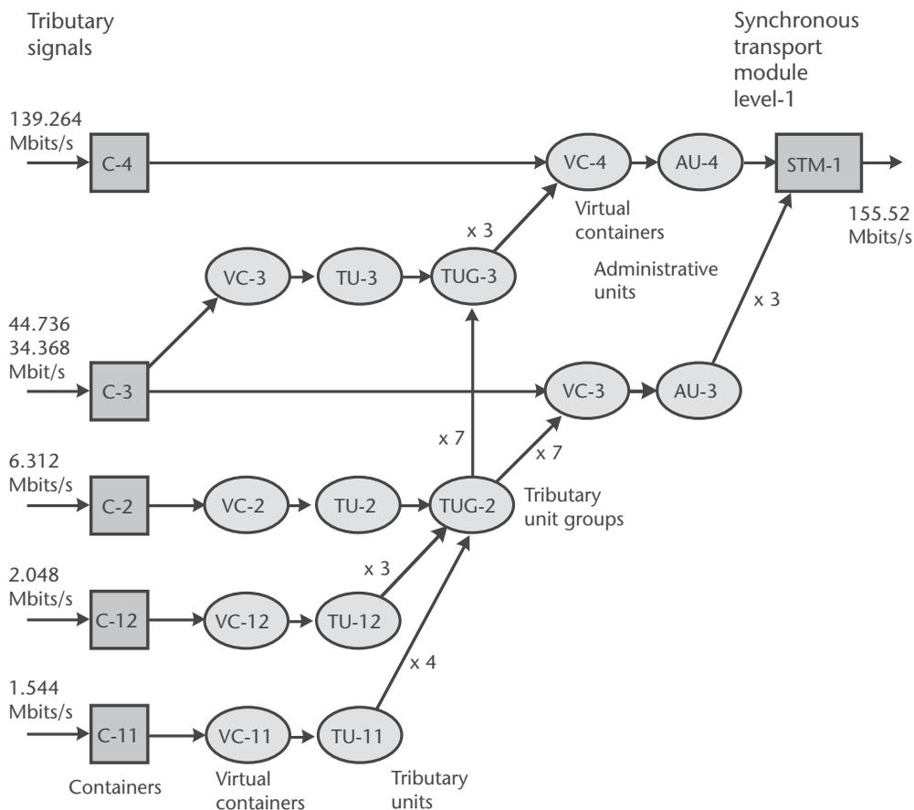
Figure 7.13 Tributary multiplexing scheme to create STM-1 frame.
