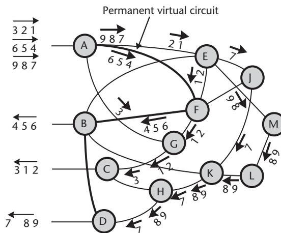
Frames 1, 2, and 3 are sent from A to C with distributed routing
