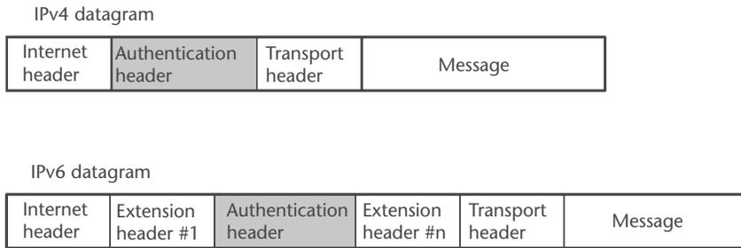
**Figure 6.6** Authentication headers in IPv4 and IPv6 datagrams.
