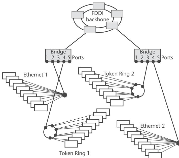
Figure 5.7 Encapsulating bridges.
