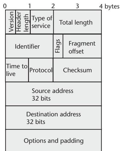
Figure 1.7 IPv4 header.
