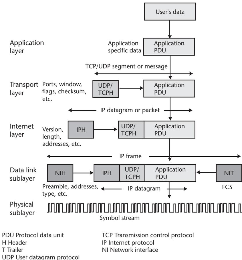
Figure 2.4 Formation of IP datagram and IP frame.
