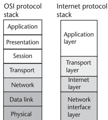
**Figure 2.3** Comparison of OSI and Internet Protocol stacks.
