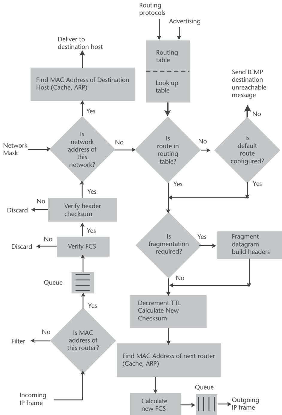
Figure 5.9 Router functions.
