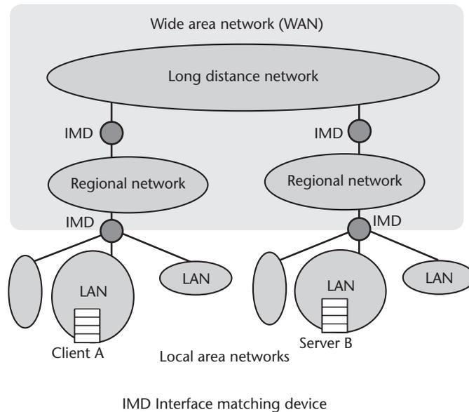
**Figure 5.1** Connecting Client A to Server B.
