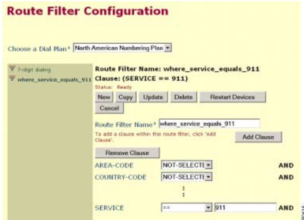
Figure 5-6 Route Filter Configuration Window
