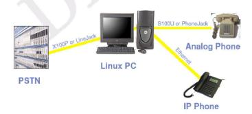
One question that is often heard is "How small of a PBX can you build with Asterisk?". Well, you can make a PBX as small as one port of PSTN and one port of analog or IP phone. Yes, it is true that you can make a PBX with just one port, but it isn't very useful unless
