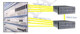
Asterisk can be used as a high density IVR and conferencing platform, using traditional PRI/T1 interfaces, and providing redundancy, scalability, and intercommunication using TDM over Ethernet, which permits Asterisk to extend the TDM bus across the ethernet network, while retaining minimal latency.
