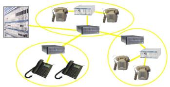
One of Asterisk's most powerful features is its ability to link remote offices of a SME (that's "Small to Medium Enterprise") together. The above diagram shows how you can build individual small PBX's for multiple offices using Asterisk, and then link them together transparently into a single network.
