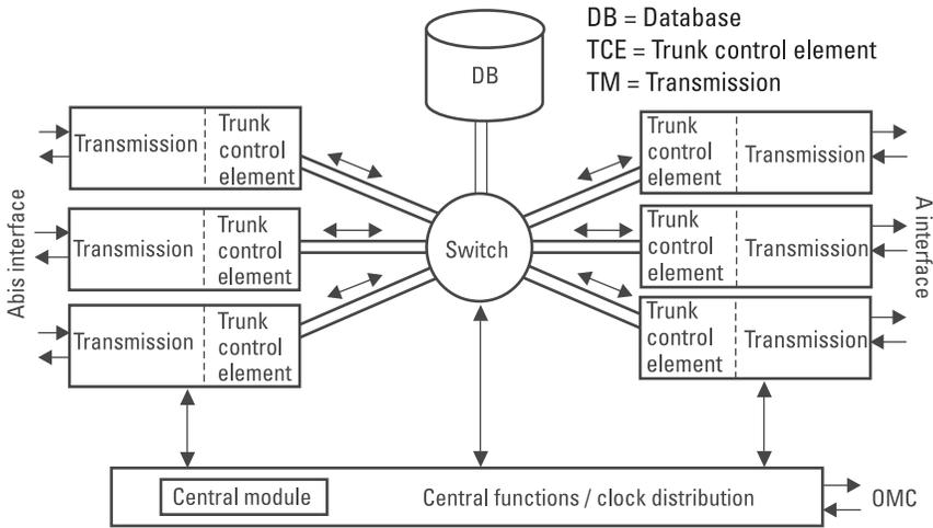
**Figure 1.3** Principal circuit diagram of the BSC.
