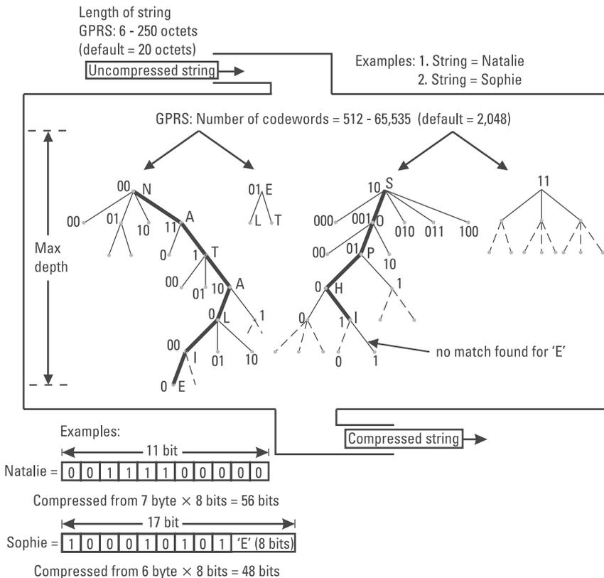
**Figure 2.18** Principles of V.42bis compression.
