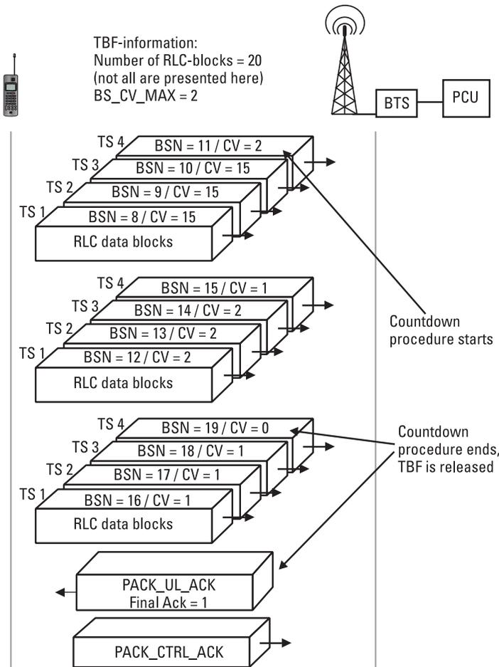
Figure 3.35 Example of the countdown procedure on one time slot.
