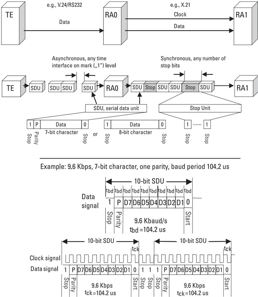
**Figure 6.20** RA0 serial data units.
