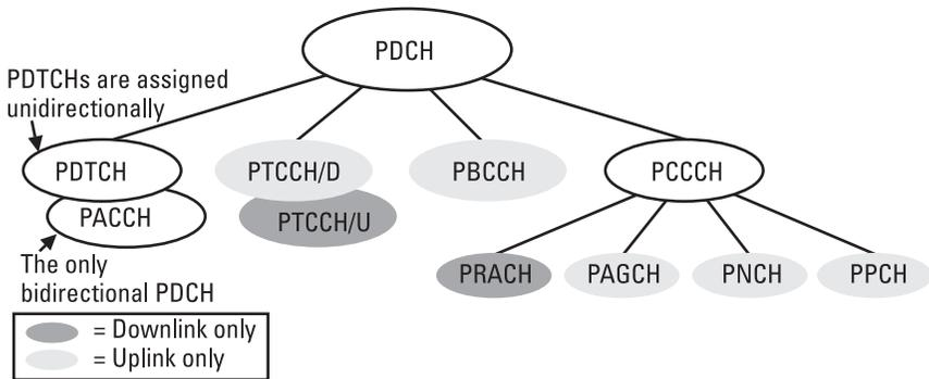
**Figure 3.4** The various packet data channels and their directional dependence.
