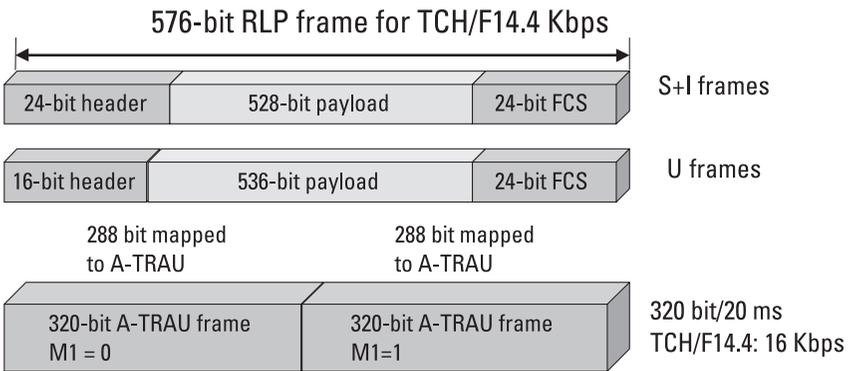
**Figure 6.37** RLP frame setup and V.110/A-TRAU mapping.
