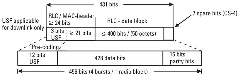
**Figure 3.18** Coding according to CS-4.
