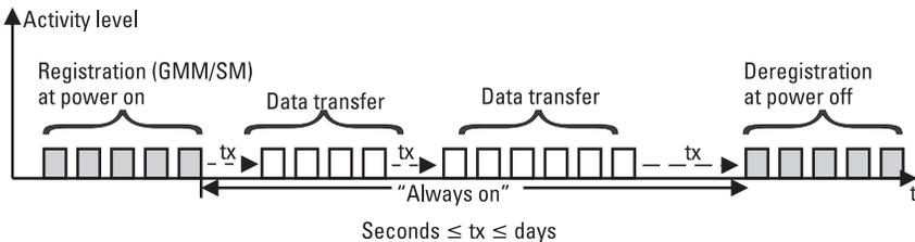
**Figure 2.10** After registration, GPRS enables the subscriber to have always-on status.
