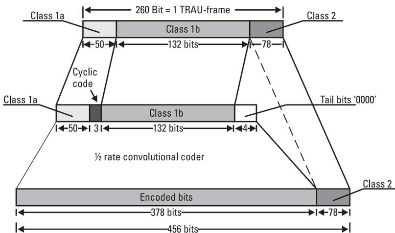
**Figure 1.23** The process of convolutional coding for FR speech.
