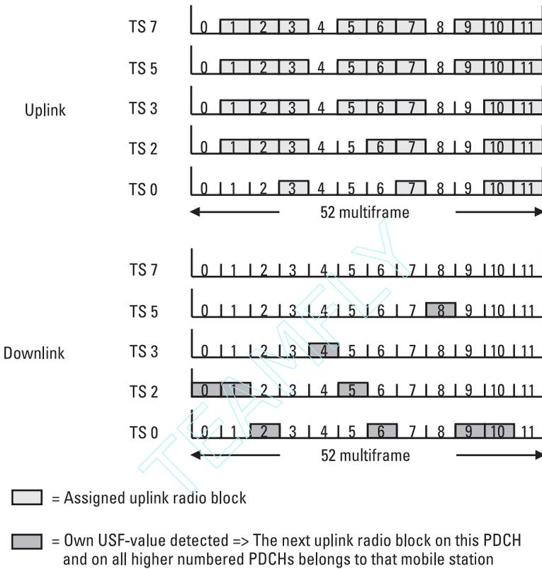
**Figure 3.31** Example of the procedures in extended dynamic allocation.
