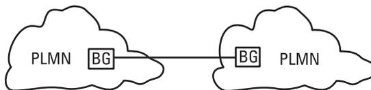
**Figure 2.22** The border gateway as a link between two PLMNs.
