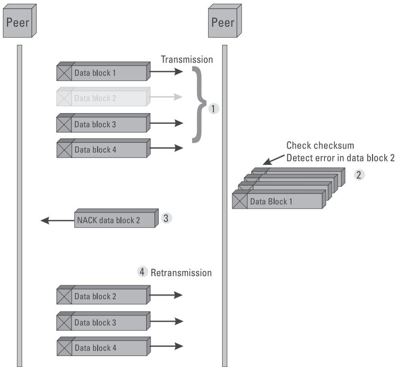
**Figure 5.4** The disadvantages of BEC.
