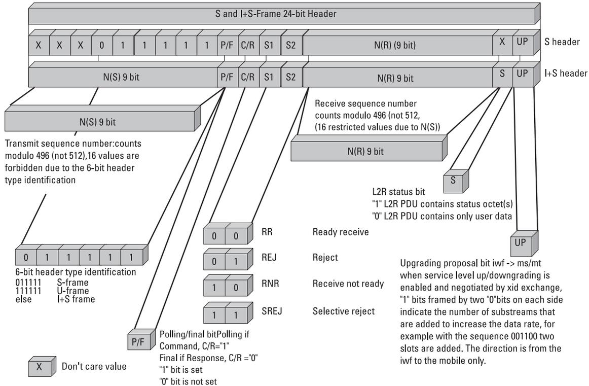
**Figure 6.39** S, I + S-frame header.
