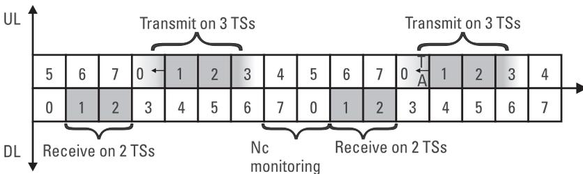
Figure 2.25 Example of the operation of a multislot class 12 with neighboring cell level measurements, taking timing advance into account. The mobile station receives on two time slots and transmits on three.
