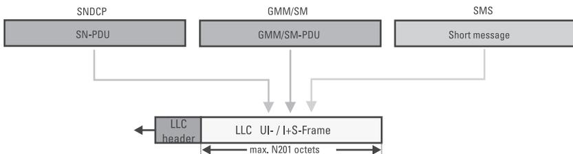
**Figure 5.14** The higher layers supply LLC with preprocessed PDUs.
