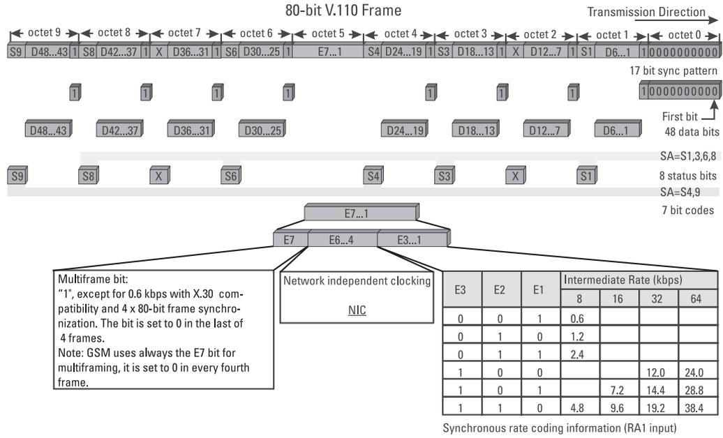
**Figure 1.40** The format of the V.110 frame/80 bits.
