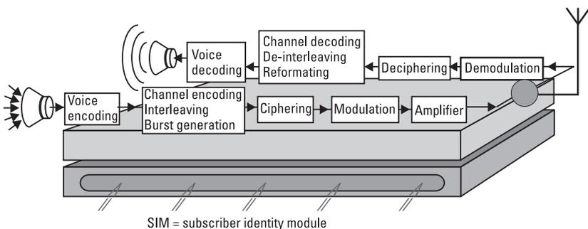
**Figure 1.7** Circuit diagram of a GSM mobile station.
