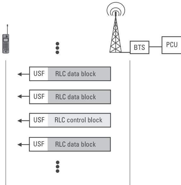
**Figure 3.28** The USF always forms the first 3 bits in every downlink RLC/MAC block.
