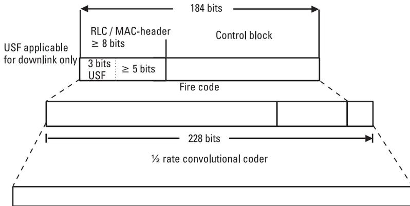
**Figure 3.16** CS-1 in the coding of RLC/MAC control messages.
