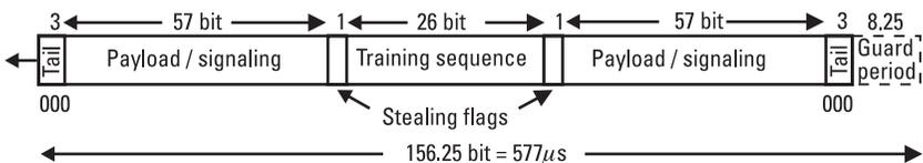
**Figure 1.34** The normal burst.
