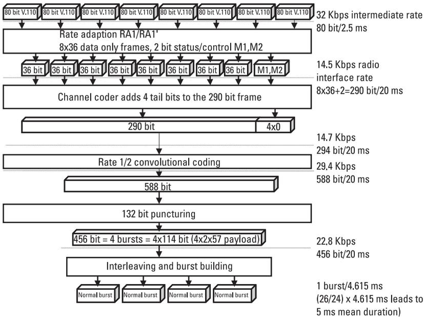
Figure 6.10 TCH/F14.4, V.110 frame air interface.
