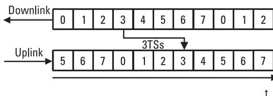
**Figure 1.12** Synchronization of downlink and uplink transmission in GSM.
