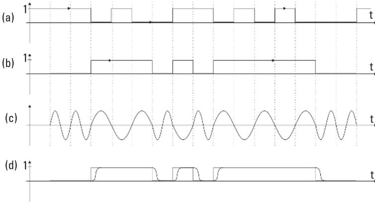
**Figure 1.35** The path from FSK to GMSK: (a) Bit stream, (b) bit stream after XOR operation, (c) MSK signal, and (d) behind Gaussian filter.
