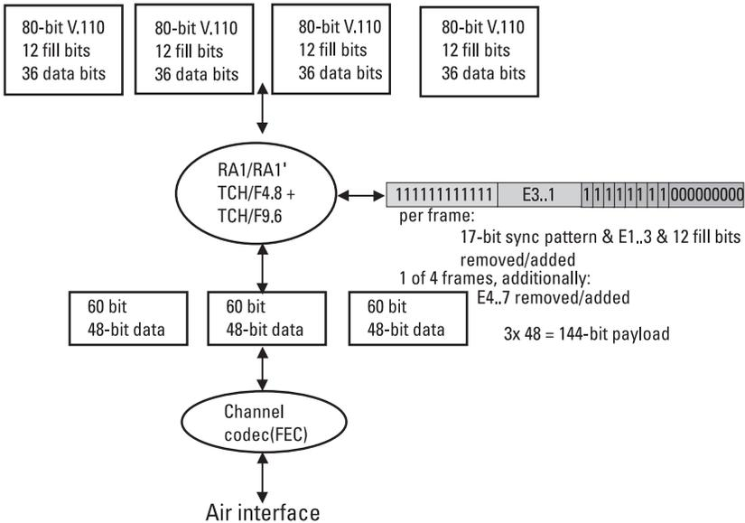
**Figure 6.25** RA1/RA1' exception for 14.4 Kbps and 28.8 Kbps.
