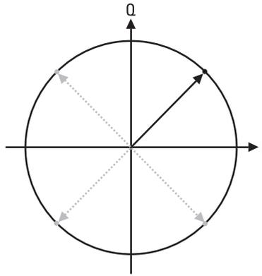
**Figure 1.36** GMSK on the I/Q level.
