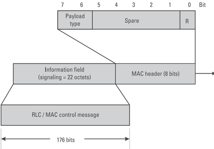
**Figure 5.10** The format of the RLC/MAC frame for uplink transfer of RLC/MAC control messages.
