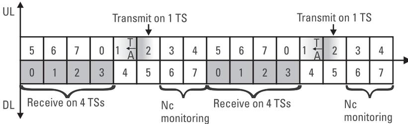
Figure 2.24 Example of the operation of a multislot class 12 with neighboring cell level measurements, taking timing advance into account. The mobile station receives on four time slots and transmits on one.
