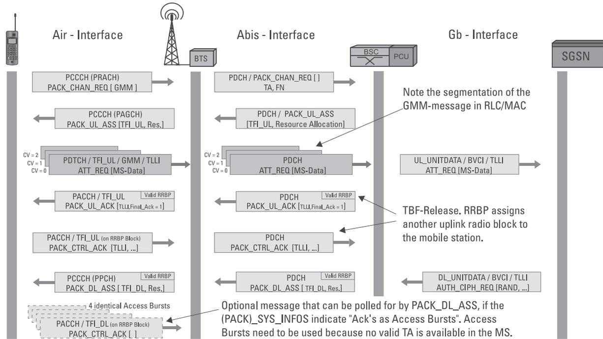
**Figure 4.7** The GPRS attach via the PCCCH.
