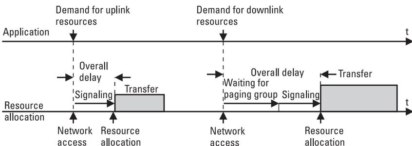
**Figure 2.11** Delay times in resource allocation in uplink and downlink directions.
