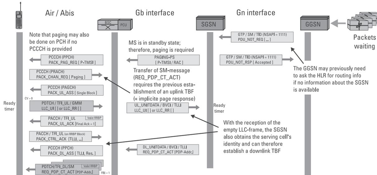
Figure 4.19 A mobile terminating PDP context activation via the PCCCH.
