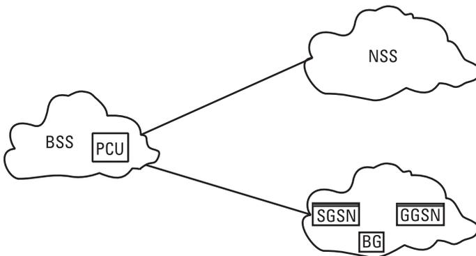
**Figure 2.13** The BSS is used equally by the NSS and the GPRS core network.
