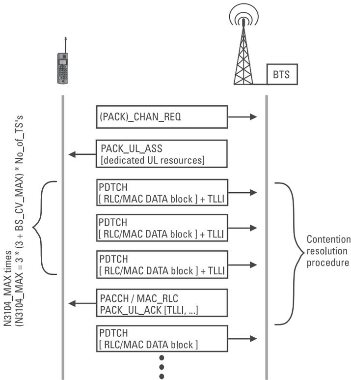
**Figure 3.22** The procedure of one-phase packet access (CCCH and PCCCH).
