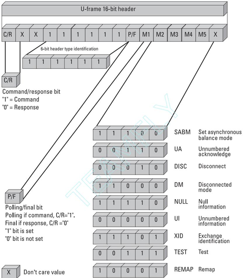
Figure 6.38 U-frame header.
