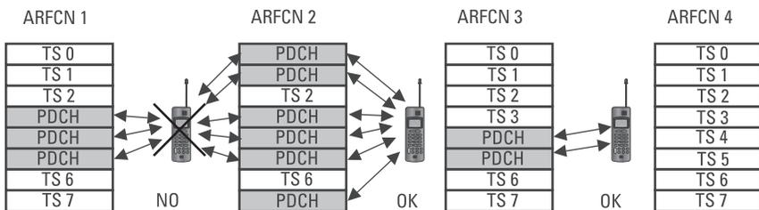
Figure 3.6 GPRS resources can only be occupied on one ARFCN.
