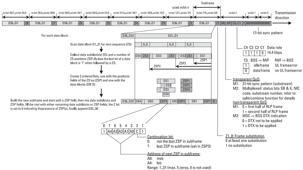
Figure 6.35 Null octet substitution with ZSP fields.
