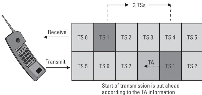
**Figure 1.13** The mobile station sets its start of transmission ahead according to the timing advance.
