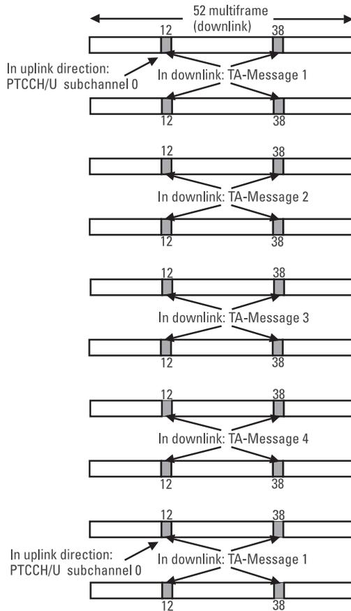
**Figure 3.12** Transmission of the new timing advance values in the timing advance messages.
