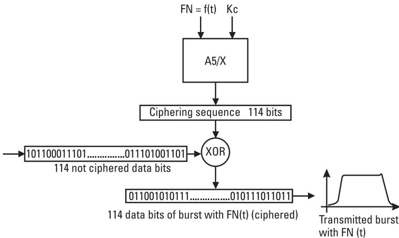
Figure 1.27 The process of data encryption in GSM.
