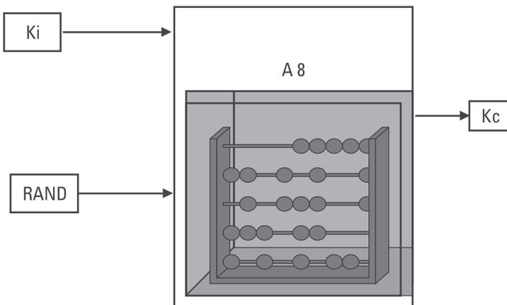
**Figure 1.5** The determination of SRES from  $K_i$  and RAND.
