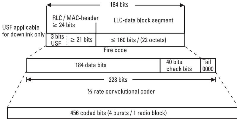
**Figure 3.15** CS-1 in the coding of LLC data.
