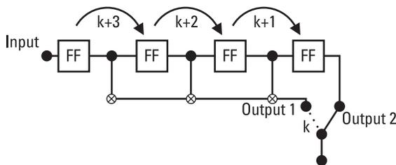
**Figure 1.24** Example of a 1:2-rate convolutional coder.
