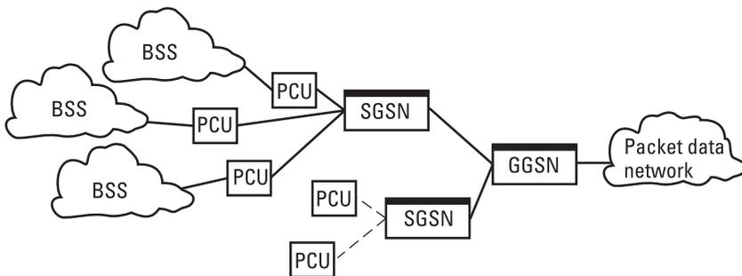
**Figure 2.16** The positioning of the SGSN in the network as a whole.
