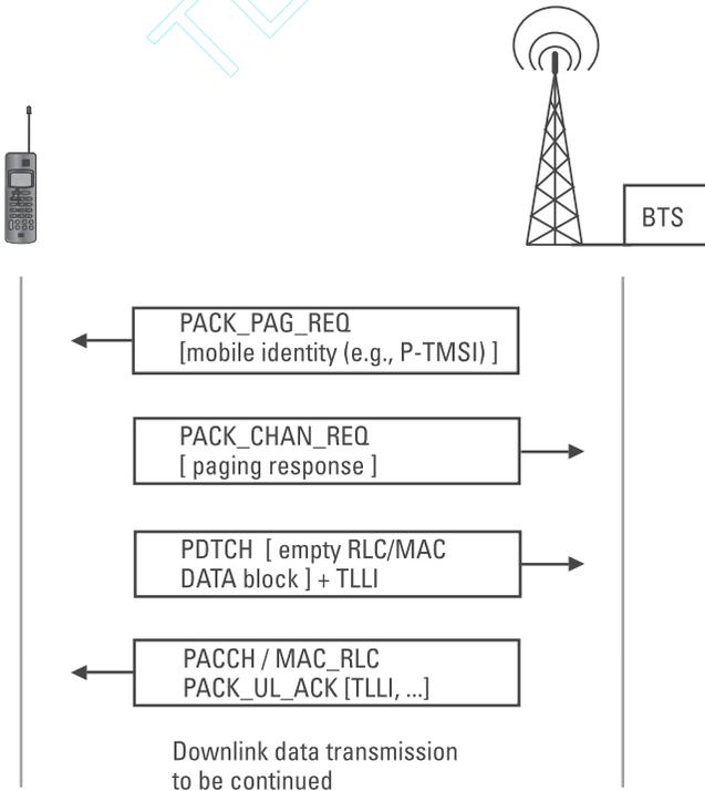
**Figure 3.25** Procedure in page response (only if PCCCH is configured).
