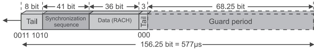
**Figure 1.33** The access burst.
