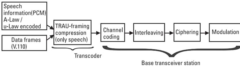
**Figure 1.21** The signal processing chain in GSM.
