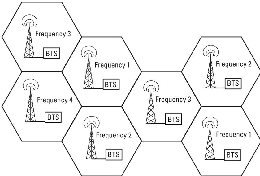
**Figure 1.8** The SDMA multiple access process gives rise to cellular network architecture.
