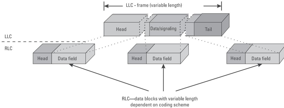
**Figure 5.3** The segmenting of LLC frames by RLC.
