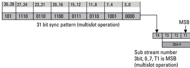
**Figure 6.31** RA1/RA1', 64 Kbps, 6 × TCH/F9.6, synchronous, transparent only.
