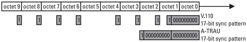
**Figure 6.34** Comparing A-TRAU and V.110 synchronization pattern.
