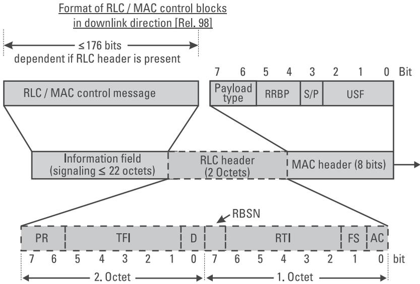
**Figure 5.9** The format of the RLC/MAC frame for downlink transfer of RLC/MAC control messages.
