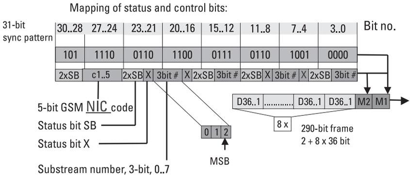
Figure 6.26 RA1/RA1', TCH14.4, data rate < 38.4 Kbps.
