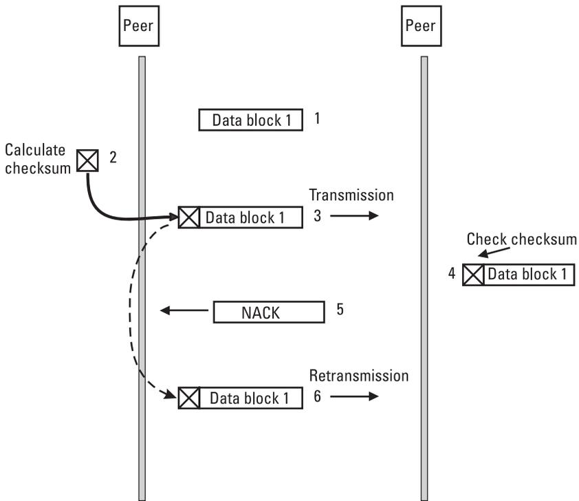
**Figure 1.22** The processes of BEC.
