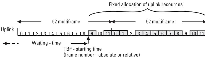
**Figure 3.27** Allocation of radio blocks using the fixed allocation method.
