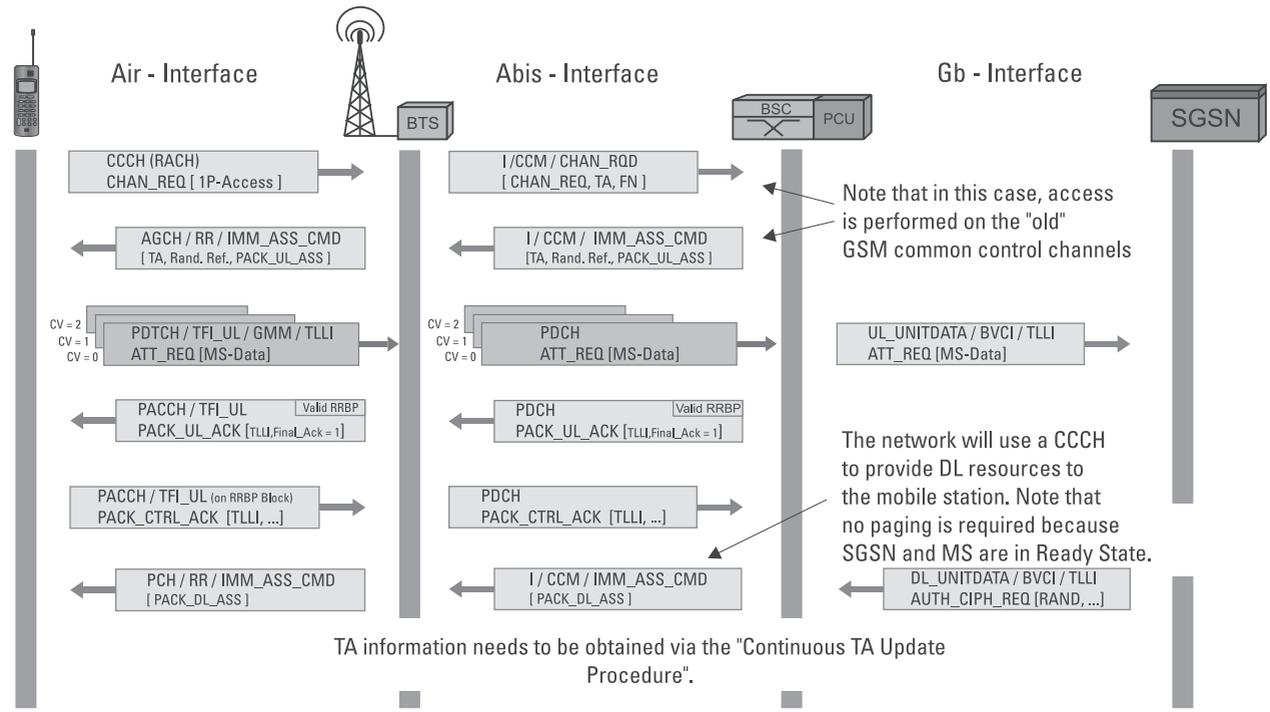
Figure 4.6 The GPRS attach via the CCCH.
