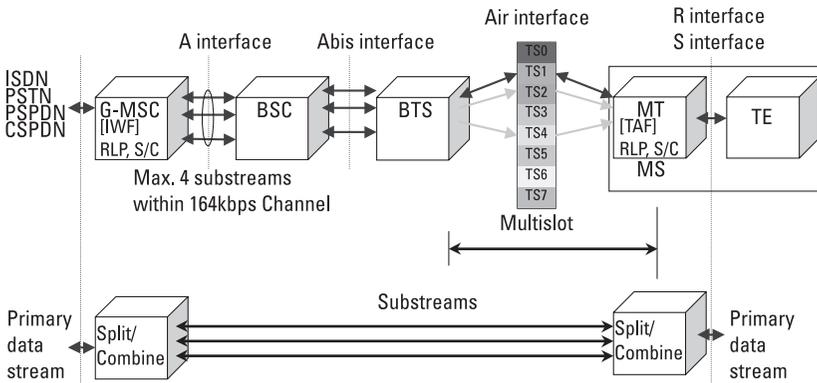
**Figure 6.1** Channel bundling in the GSM PLMN.
