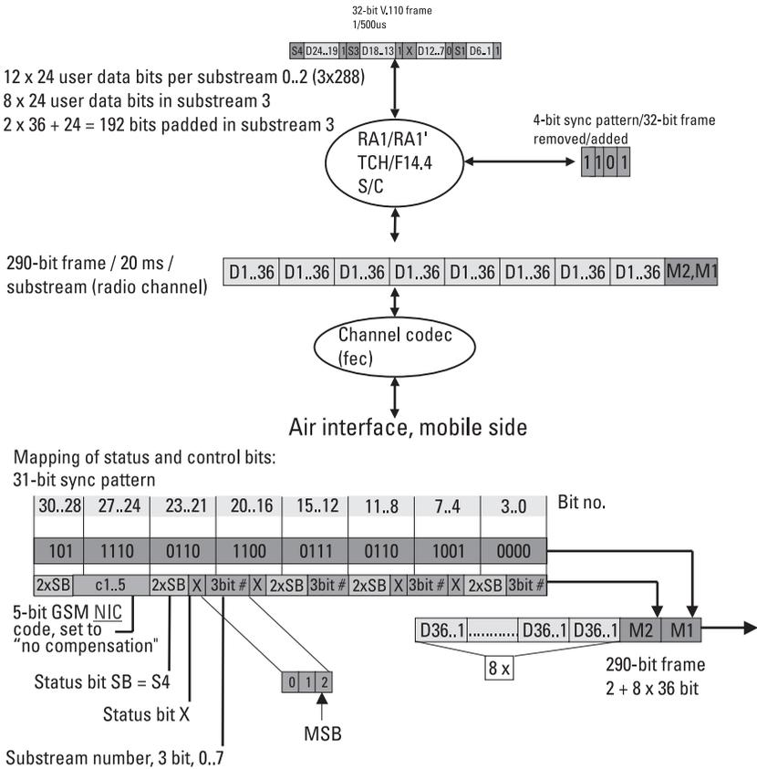
**Figure 6.28** RA1/RA1', TCH/F14.4, 48 Kbps, synchronous.
