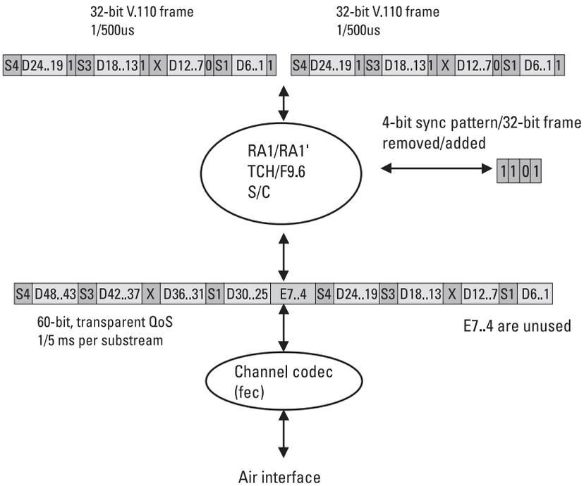
**Figure 6.27** RA1/RA1', TCH/F9.6, 48 Kbps, synchronous.
