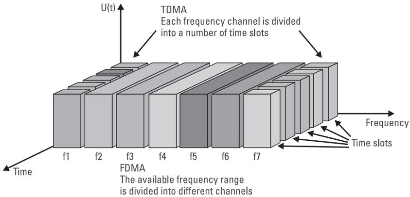
**Figure 1.10** The combination of FDMA and TDMA.
