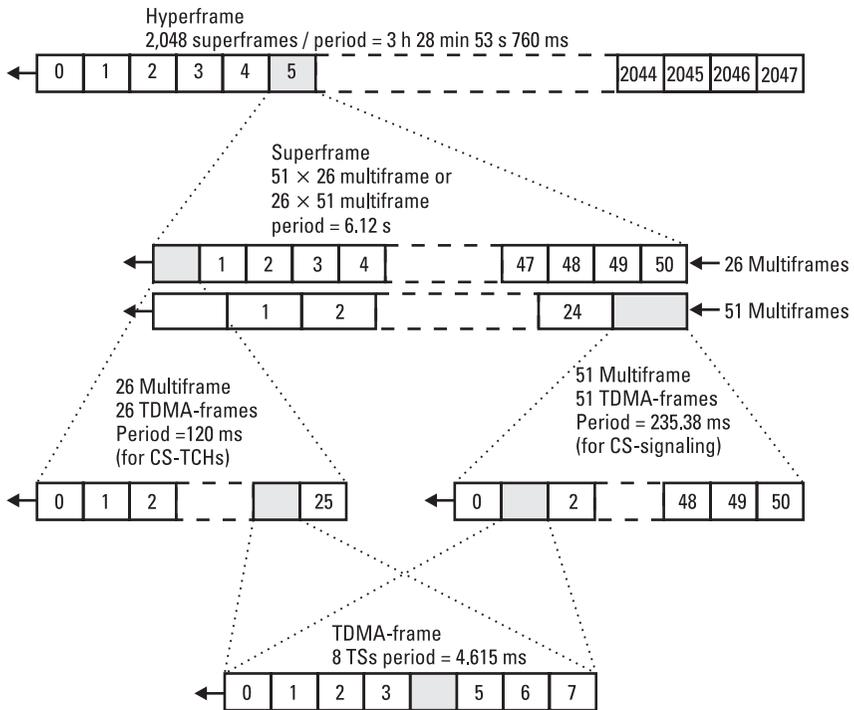
**Figure 1.20** The frame hierarchy in GSM.
