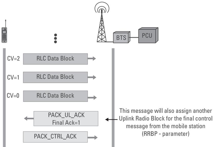
**Figure 3.34** Simplified presentation of the countdown procedure.
