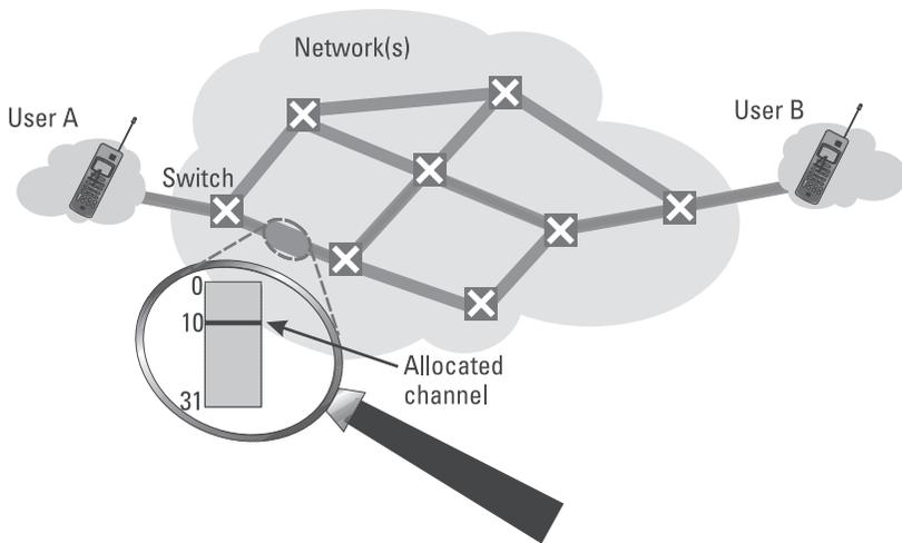
**Figure 2.4** The principle of circuit switching.
