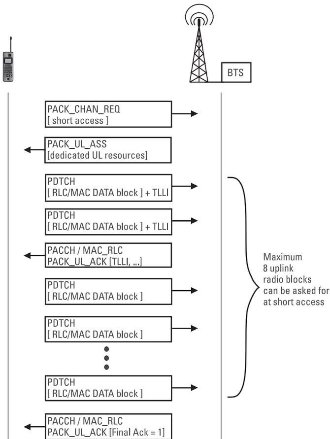
**Figure 3.24** Procedures in short access (only if PCCCH is configured).
