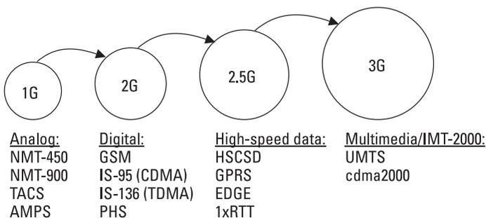
**Figure 2.1** Mobile communications generations 1 to 3.
