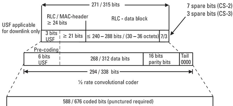
Figure 3.17 Channel coding according to CS-2 and CS-3.
