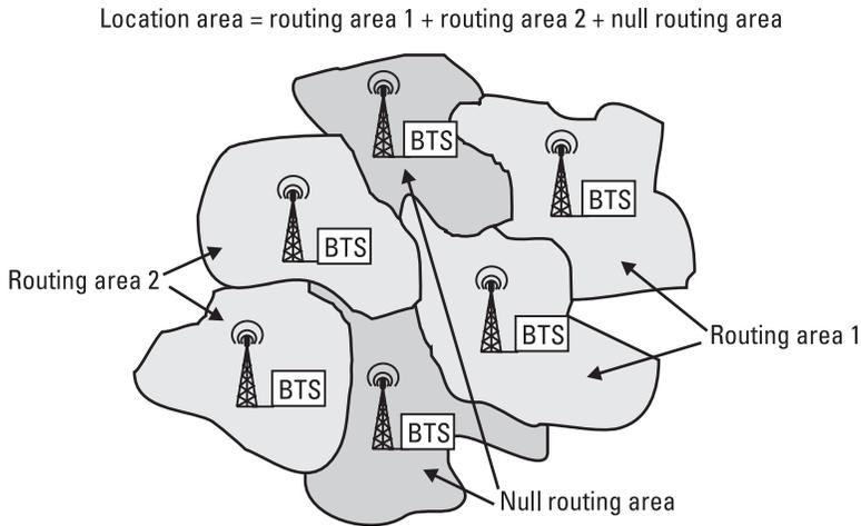
**Figure 4.5** The connections between location area, routing area, and null routing area.
