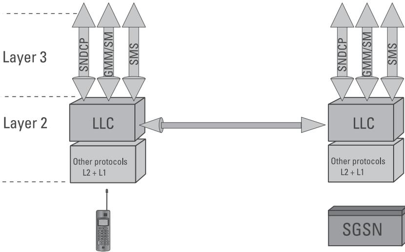
**Figure 5.13** The LLC protocol between mobile station and SGSN.
