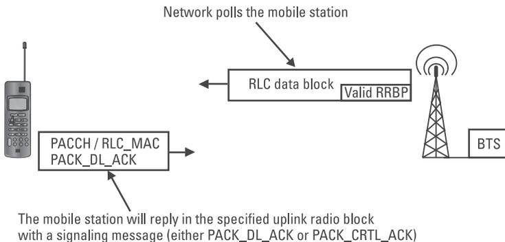
**Figure 3.32** Allocation of resources for the uplink PACCH.
