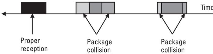
**Figure 2.8** Collisions of uplink data packets in the Aloha system.
