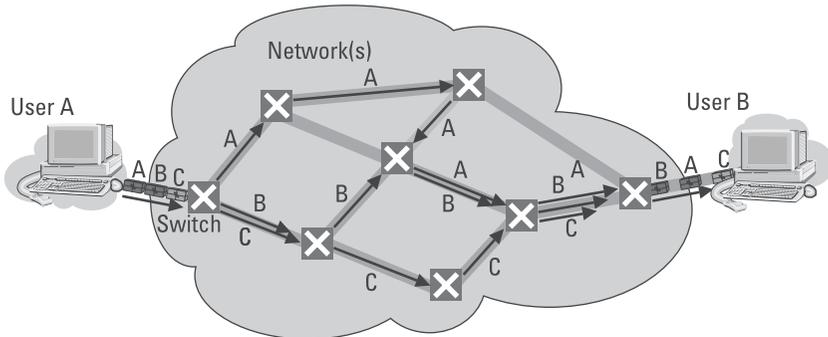
**Figure 2.5** The principle of packet switching.
