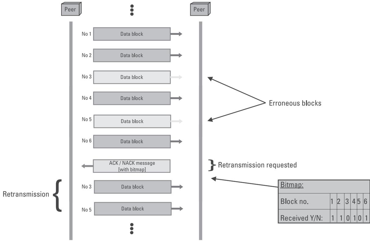
Figure 5.5 The procedures of BEC aided by ARQ.
