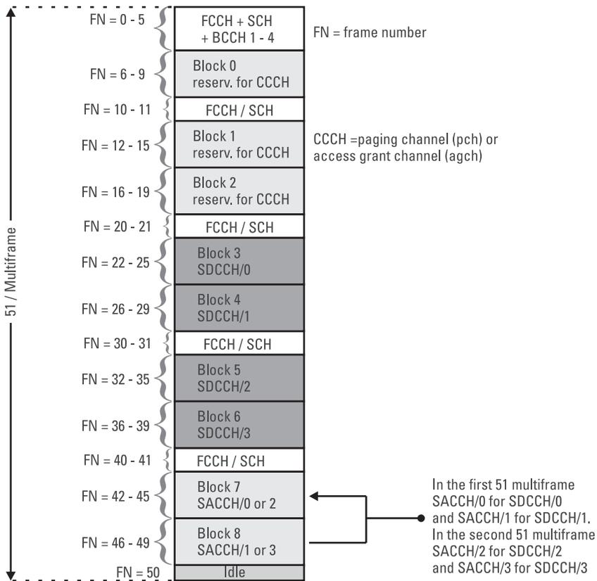
**Figure 1.18** Example of a 51 multiframe with a duration of 235.38 ms in the downlink direction of time slot 0 of a BCCH carrier.
