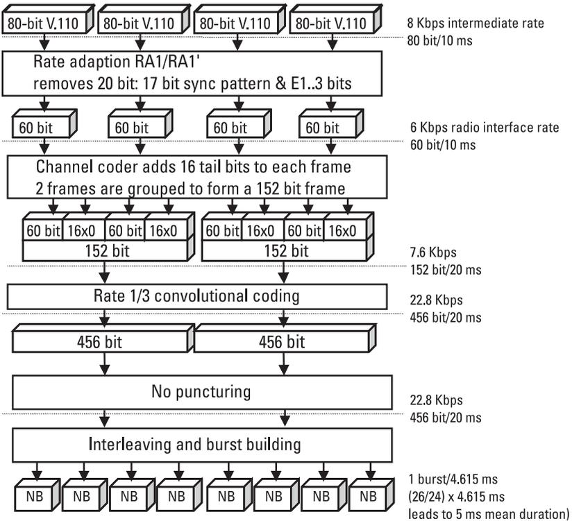
**Figure 6.9** TCH/F4.8, V.110 frame air interface.
