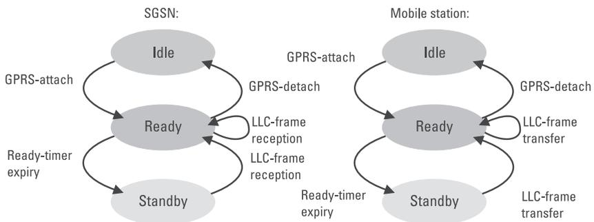
**Figure 4.15** GMM status in mobile station and SGSN.
