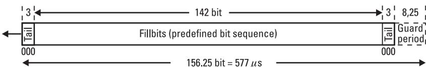
**Figure 1.31** The dummy burst.
