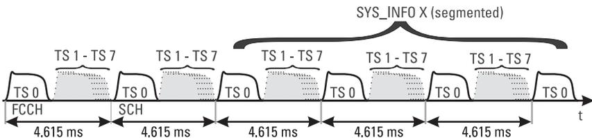
**Figure 1.17** The chronological sequence of logical channels (using time slot 0 of the BCCH carrier as an example).
