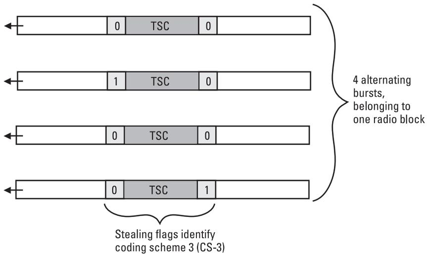
**Figure 3.19** The stealing flags in the new function of identifying the coding scheme.
