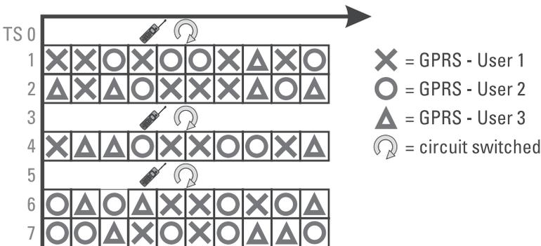
Figure 3.3 Example of resource sharing of GSM and GPRS on an ARFCN.
