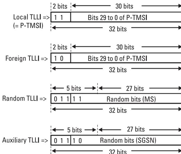
**Figure 4.3** The different types of TLLIs.
