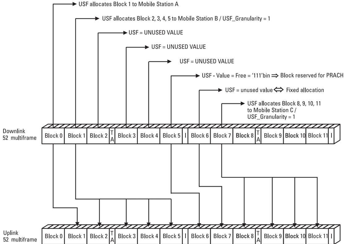
**Figure 3.30** Example of the operation of the USF on a time slot with PCCCH and fixed allocation.
