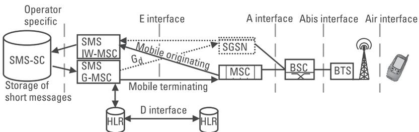
**Figure 1.38** The transmission of short messages in a combined GSM/GPRS network.
