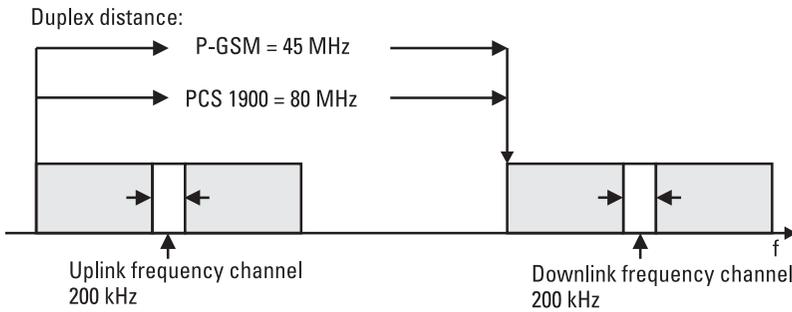
**Figure 1.9** There is a set distance between the uplink and downlink channels in the application of FDMA in GSM.
