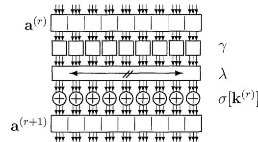
Fig. 9.1. Steps of an example block cipher.
