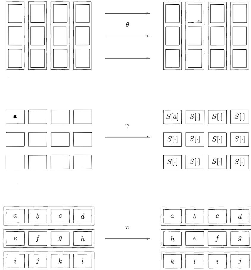
**Fig. 11.2.** The basic operations of BKSQ.  $\theta$  is a mixing step with 4 parallel linear transformations.  $\gamma$  consists of 12 separate substitutions.  $\pi$  is a shift of the rows.
