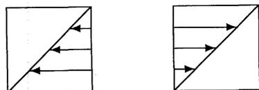
**Fig. 3.5.** Pictograms for ShiftRows (left) and InvShiftRows (right).
