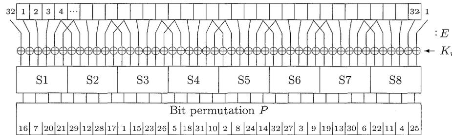
Fig. 6.2. Computational graph of the DES  $F$ -function.
