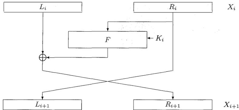
Fig. 6.1. Computational graph of the DES round function.
