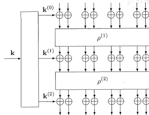
Fig. 2.7. Key-alternating block cipher with two rounds.
