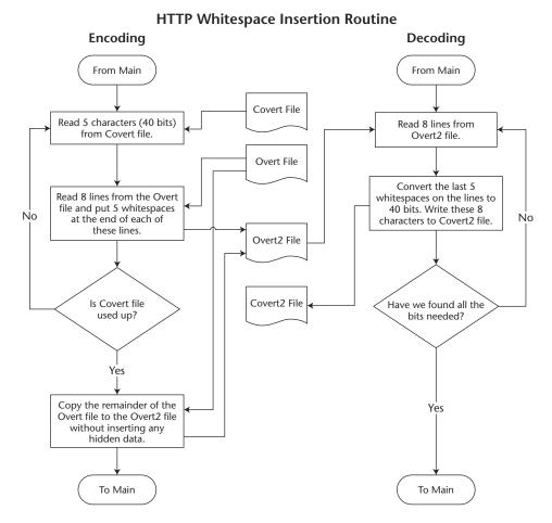
In this routine, bits are encoded as whitespaces at the end of the line in the html code. Whitespaces will not show up when the Overt2 file is viewed in a web browser. A zero is encoded as a space. A '1' bit is encoded as a tab.
