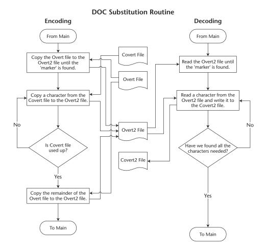
The Overt file must be a MS Word document with a special 'marker' typed into the Comment field on the document Properties window.
