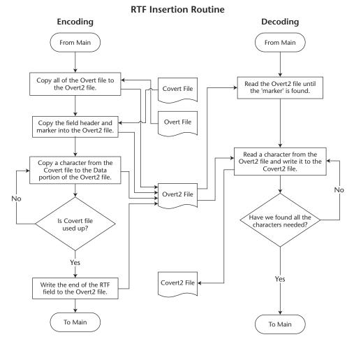
The covert data is stored in a non-printing field of the RTF file. Additionally, the data is put at the end of the RTF file, which may cause it to not display, also.
