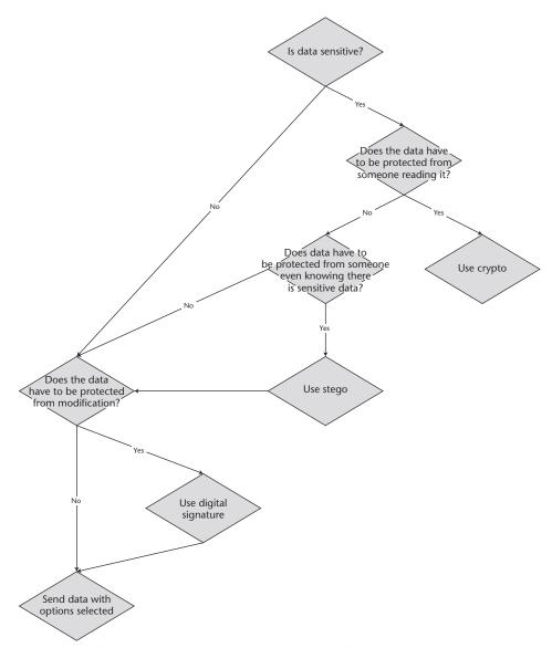
Figure 9.1 Flow chart for the secure communication decision process.
