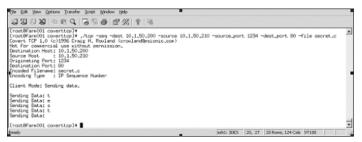
Figure 7.23 Sending data in the TCP header.
