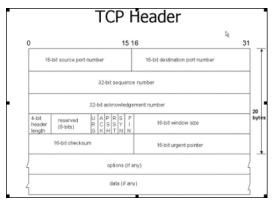
Figure 7.18 TCP header.
