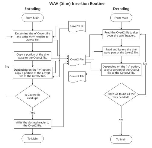
This algorithm creates a crude sine wave in the data portion of the Overt2 WAV file. Depending on the command line argument "-v <2|4|8>", either half, one-quarter, or one-eighth of the sine wave data is replaced with the covert data.
