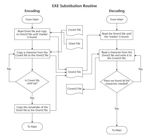
The Overt executable file must compile in the routine 'exe\_marker.c' in order to save the space in the exe file to hide the covert data. When this module is compiled in, there is enough space in the exe file to hold the covert data.
