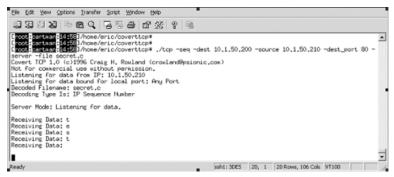
Figure 7.24 System receiving data that is hidden in the TCP header.
