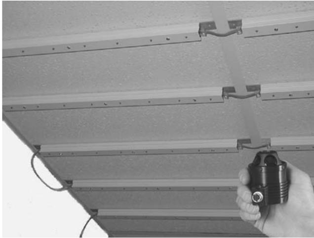
**Figure 17.4** The HiBall optical tracker. © 3rdTech. Reprinted by permission
