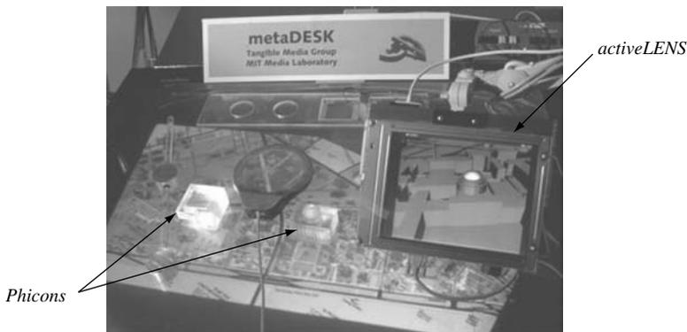
**Figure 17.5** The metaDESK system. From (Ishii and Ullmer 1997). © 1997 ACM Inc. Reprinted by permission
