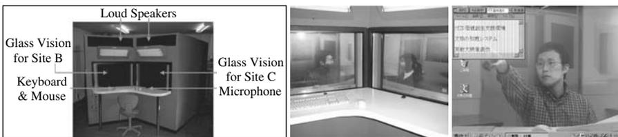
**Figure 5.8** MONJUnoCHIE: the system name originates from a Japanese proverb meaning that two is better than one. *Left*: terminal for a three-party connection. *Middle*: image of a running session. *Right*: HOE display with touch screen sensors. Reproduced by permission of Yasuda-Aoki-Laboratory, Research Center for Advanced Science and Technology (RCAST), University of Tokyo (Aoki *et al.* 1999)
