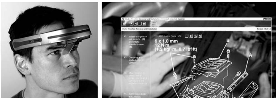
**Figure 14.1** By superimposing test and repair data into vision, the Nomad Augmented Vision System allows reading detailed service information and following complex instructions directly at the point of task (Reproduced by permission of Microvision Incorporated)
