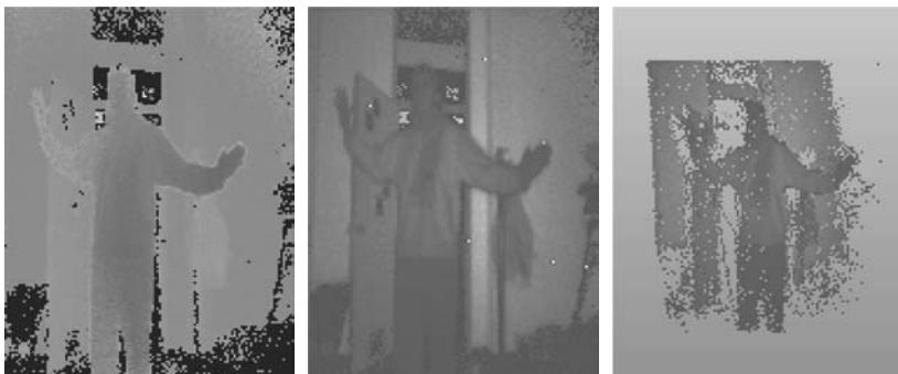
**Figure 16.14** Snapshot of a real time (20 frames/s) scan of a person: (a) grey level; (b) reflectance; (c) 3D perspective view (124 × 160 points, for a field of view of 42 × 46°)
