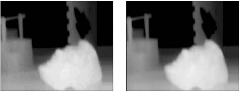
**Figure 2.7** Comparison of coding artifacts for ‘Orbi’ test sequence. Roughly the same bitrate of about 145 kbit/s was used for both codecs. (1) Rate-distortion (R/D) optimized MPEG-4 Visual codec - 37.74 dB (QP30); (2) AVC codec - 45.35 dB (QP30)
