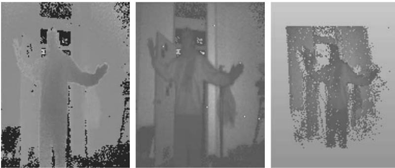
**Figure 16.14** Snapshot of a real time (20 frames/s) scan of a person: (a) grey level; (b) reflectance; (c) 3D perspective view ( $124 \times 160$  points, for a field of view of  $42 \times 46^\circ$ )
