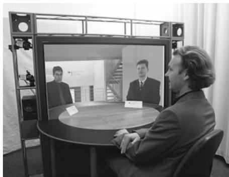
**Figure 11.10** Immersive virtual environment video conference setup at Fraunhofer HHI, Berlin. In this scenario persons from different remote locations are arranged around a virtual table. Each participant can be compressed as an arbitrarily shaped video object using the MPEG-4 object-based coding modes (Tanger *et al.* 2004)
