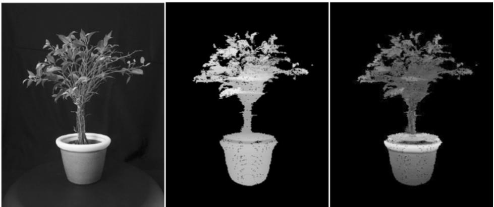
**Figure 8.16** ICT reconstruction of the *Tree* sequence. *Left*: original frame of a tree on a turntable. *Middle*: reconstructed geometry displayed as depth map. *Right*: synthesized image from the voxel volume
