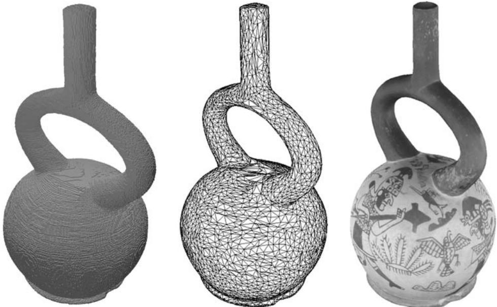
**Figure 8.4** *Left:* voxel volume of a Peruvian vase reconstructed from 72 images. *Middle:* triangle mesh derived from the voxel volume. *Right:* textured 3D model
