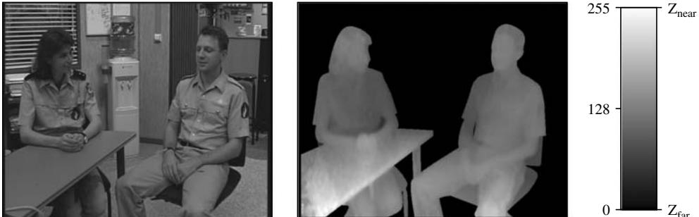
**Figure 2.3** The ATTEST data representation format consisting of: (1) regular 2D colour video in digital TV format; (2) accompanying 8-bit depth-images with the same spatio-temporal resolution
