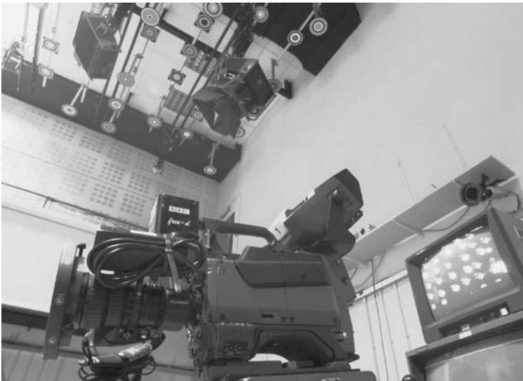
**Figure 3.1** The BBC ‘Free-D’ camera tracking system is based on circular bar-coded targets on the ceiling and an auxiliary camera looking upwards. Real-time hardware computes the position and orientation of the camera at a 50 Hz update rate
