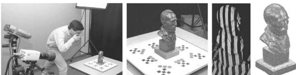
**Figure 4.11** Data acquisition process (Reproduced by permission of the ACM from Chen *et al.* 2002): (a) capturing many images; (b) sample image; (c) painted object; (d) 3D triangular mesh
