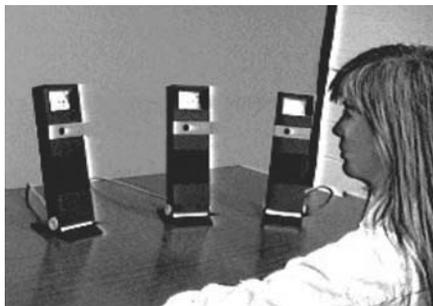
**Figure 5.6** The Hydra concept: a local user is sitting in front of three Hydra units, substituting the remote conferees physically. Each unit consists of its own camera, monitor and loudspeaker. Reproduced by permission of William Buxton (Snellen and Buxton 1992)
