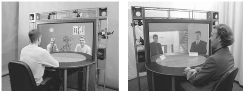
**Figure 5.12** Semi-immersive videoconferencing on its way to the market. *Left*: the experimental system of the European IST project VIRTUE using a 61-inch plasma display. *Right*: the immersive meeting point (im.point), a follow-up prototype of VIRTUE using a MPEG-4-based software implementation and standard PC technology
