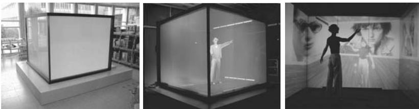
**Figure 5.14** Blue-C: an immersive portal for tele-collaboration. *Left:* the CAVE-like construction of blue-C. *Middle:* outside view of a blue-C session while active screen is transparent. *Right:* inside view while active screen is opaque (shop application). Reproduced by permission of the blue-C project, ETH Zürich, Switzerland
