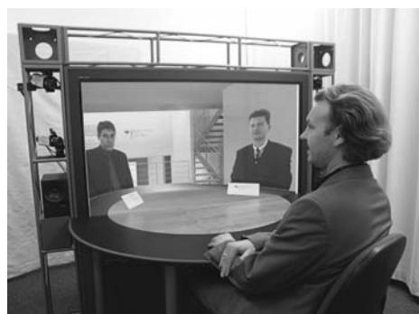
**Figure 11.10** Immersive virtual environment video conference setup at Fraunhofer HHI, Berlin. In this scenario persons from different remote locations are arranged around a virtual table. Each participant can be compressed as an arbitrarily shaped video object using the MPEG-4 object-based coding modes (Tanger *et al.* 2004)
