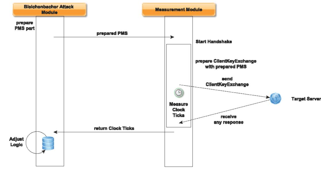
Timing measurements with a patched version of the TLS implementation **MatrixSSL**
