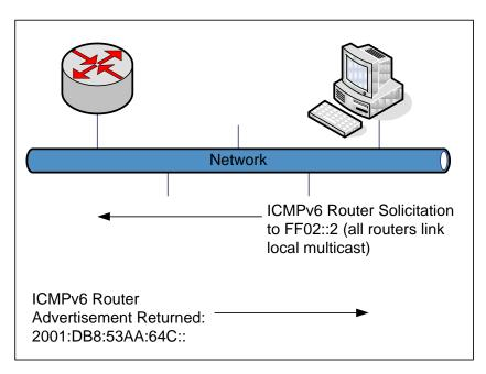
Figure 3-12. Example of Stateless Address Autoconfiguration (SLAAC)
