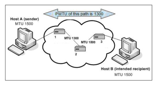
Figure 3-13. Significance of MTU under IPv6
