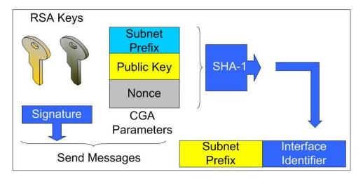
Figure 5-2. Generating Cryptographic Addresses from Public-Private Key Pairs
