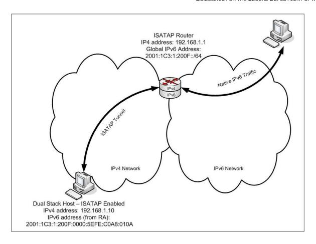
Figure 6-3. Example - Tunneling IPv6 over IPv4 Networks with ISATAP
