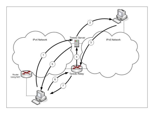
Figure 6-4. Example - Tunneling IPv6 over IPv4 Networks with Teredo
