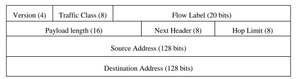
Figure 3-6. The IPv6 Packet Header Format (Field Sizes in Bits) (RFC 2460)
