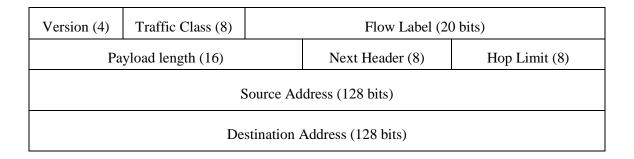
Figure 2-1. The IPv6 Packet Header Format (Field Sizes in Bits)<sup>7</sup>
