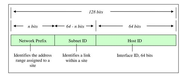
Figure 3-1. IPv6 Address Format
