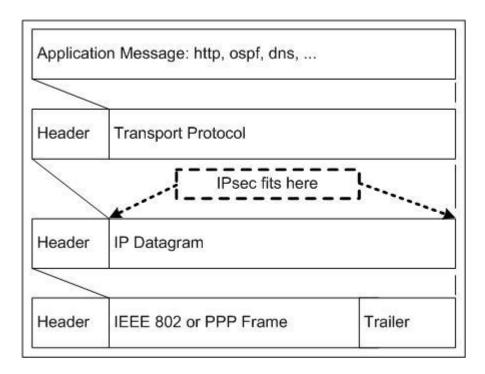
Figure 5-3. IPsec in the TCP/IP Protocol Stack
