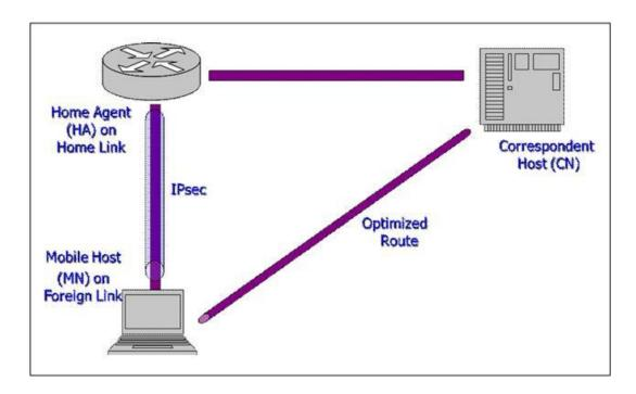
Figure 4-2. The Main MIPv6 Components
