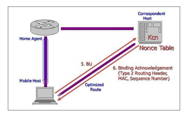
Figure 4-7. Reverse Routability—BU and BUA Protected with Kbm
