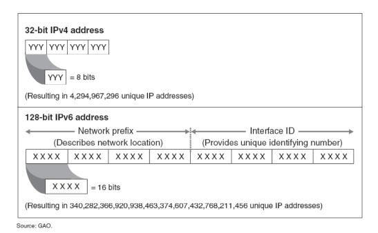
Figure 3-5. A Comparison of IPv4 and IPv6 Addressing<sup>7</sup>
