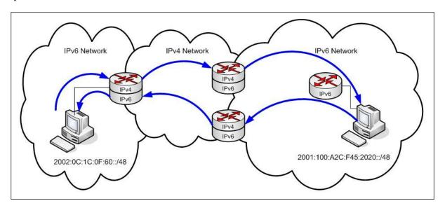
Figure 6-1. Example of Tunneling IPv6 over IPv4 Networks
