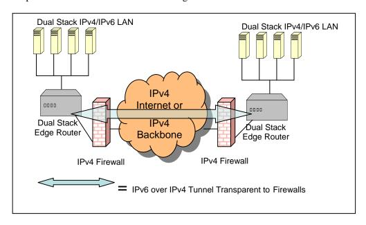
Figure 6-2. IPv6 over IPv4 Tunnels Transparent to the IPv4 Infrastructure
