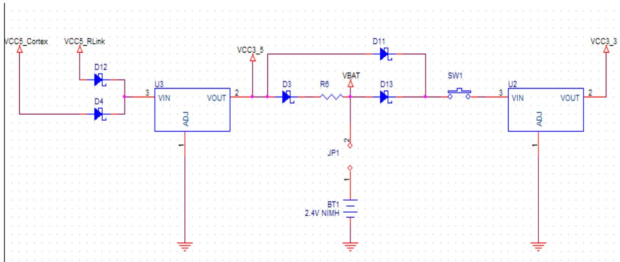
When one USB connector is linked to a PC host (either the RLink or the STM32), the 5V voltage supplied by the PC is used to recharge the batteries.
