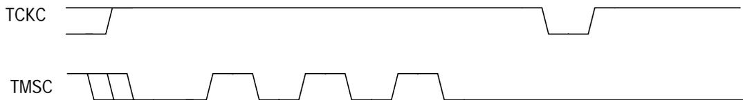
As described in the IEEE Specification, there may be a TMSK edge coincident with the last rising edge of TCKC before the Escape sequence begins, and that edge may or may not be detected by the Escape logic, depending on signal skew. A single pulse that would normally be two edges could therefore be counted as three edges. Escape detection logic takes this possibility into account. The Adapter interprets TMSK edges in an Escape as described in the following subsection.
