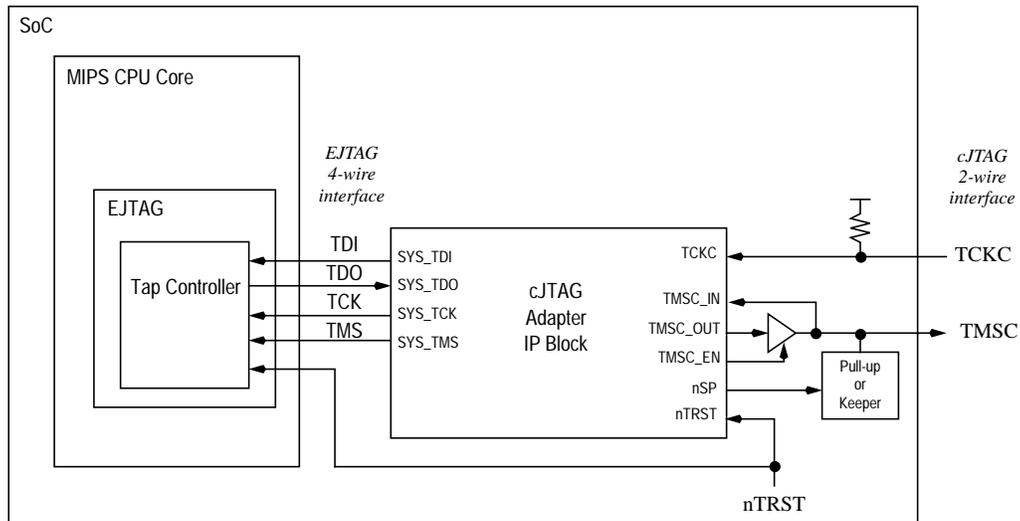
The clock of cJTAG (*TCKC*) interface and EJTAG (*SYS\_TCK*) interface operate synchronously with a 3X speed ratio as shown in Figure 6. *SYS\_TCK* is generated based on *TCKC* inside the cJTAG block by masking out 2 of the pulses every 3 cycles. It is important to constrain *TCKC* with a 3X frequency as the normal clock will run in the EJTAG block.
