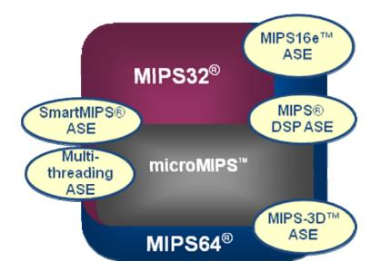
MIPS also previously developed an extension called MIPS16e<sup>™</sup> that was designed to minimize code size and thus the memory required in an application. MIPS16e introduced a number of 16-bit instructions that could be used in place of the standard 32-bit instructions with the goal of minimizing system cost. We'll get to the specifics of the new microMIPS ISA shortly, and how it improves on the MIPS16e effort.
