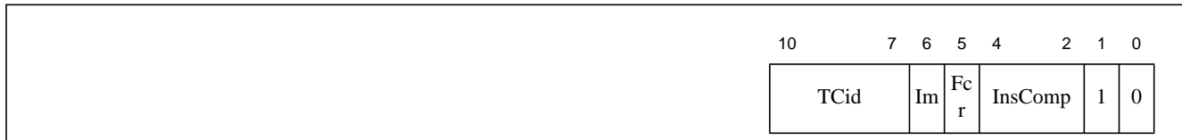
Figure 4.12 TF2 with Optional Bits and TCid Bits (Trace Format 2 Single-Pipe)
