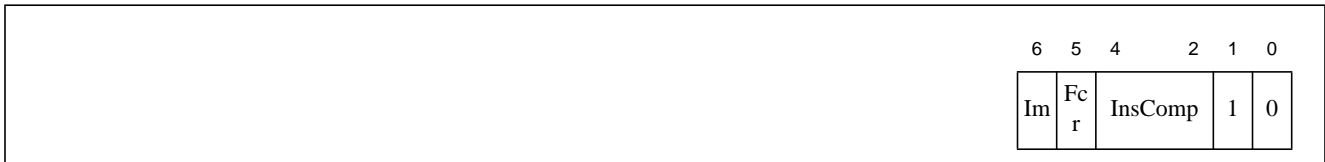
Figure 4.3 TF2 with Optional Bits (Trace Format 2 Single-Pipe)
