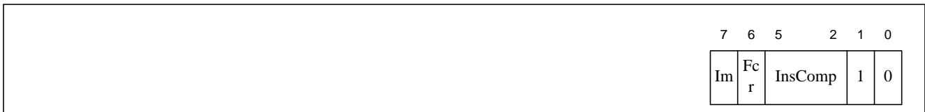
Figure A.2 Expanded TF2 with Optional Bits (Trace Format 2 Single-Pipe)
