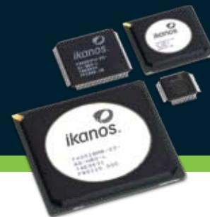
The Fx™ 100100-5 and Fx10050-5 chipsets are the industry's first IPTV-optimized multi-mode (VDSL2, VDSL, ADSL2+, ADSL2 and ADSL) solutions for central office (CO) equipment (DSLAMs, ONUs and other broadband concentrators). Both chipsets support all 8, 12 and 17 MHz profiles. The Fx100100-5 chipset additionally supports the 30 MHz profile. The chipsets also support the VDSL, ADSL2+, ADSL2 and ADSL standards.
