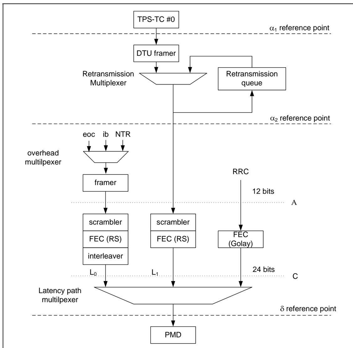
In **Figure 6**, the retransmission queue is shown at the  $\alpha$ -interface. This buffer and the DTU framer function can also be located above the  $\gamma$ -interface without disturbing the reference model.
