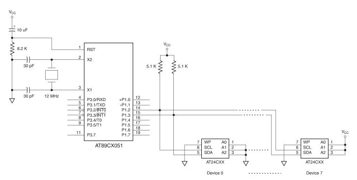
common 2-wire bus. The bus consists of a serial clock (SCL) line and a serial data (SDA) line. The clock is generated by the bus master and data is transmitted serially on the data line, most significant bit first, synchronized to the clock. The protocol supports bidirectional data transfers in 8-bit bytes.
