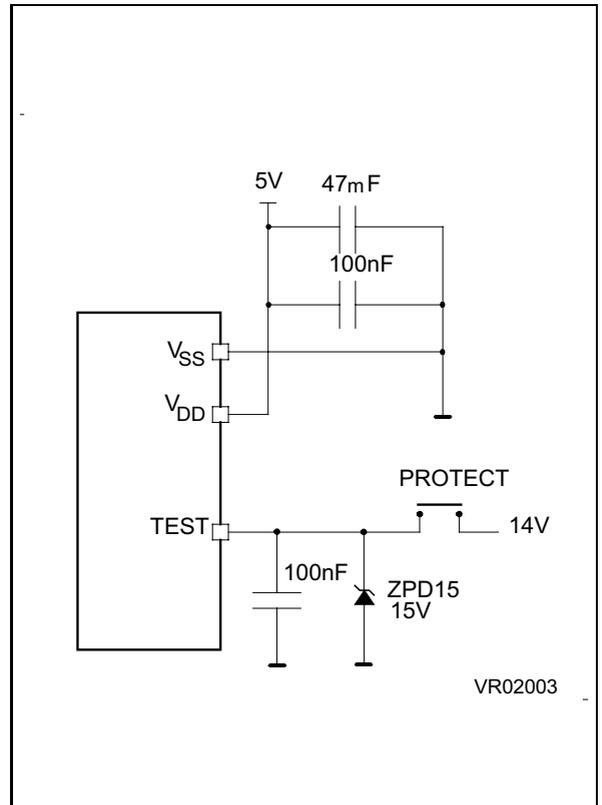
Note: ZPD15 is used for overvoltage protection
