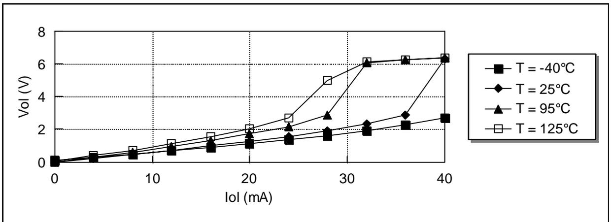
Figure 36. Vol versus Iol on all I/O port at T=25°C
