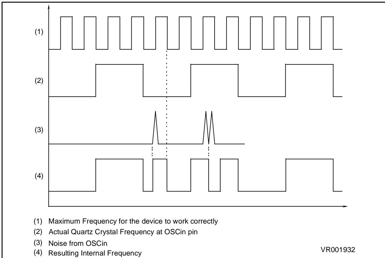
Figure 10. OSG Emergency Oscillator Principle
