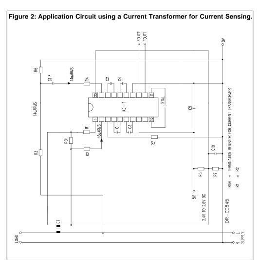
Note: Capacitor C11 may be selected for phase compensation and DC blocking.
