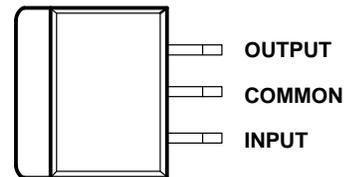
The common terminal is in electrical contact with the mounting base.
