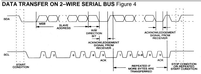
Figure 5 details how data transfer is accomplished on the two–wire bus. Depending upon the state of the R/W bit, two types of data transfer are possible:
