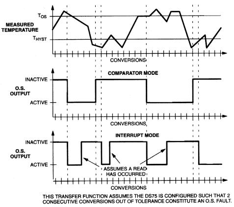
Regardless of the mode chosen, the O.S. output is open-drain and the active state is set in the configuration register. The power-up default is active low. Refer to the "OPERATION-Programming" section for instructions in adjusting the thermostat setpoints, thermostat mode, and O.S. active state.
