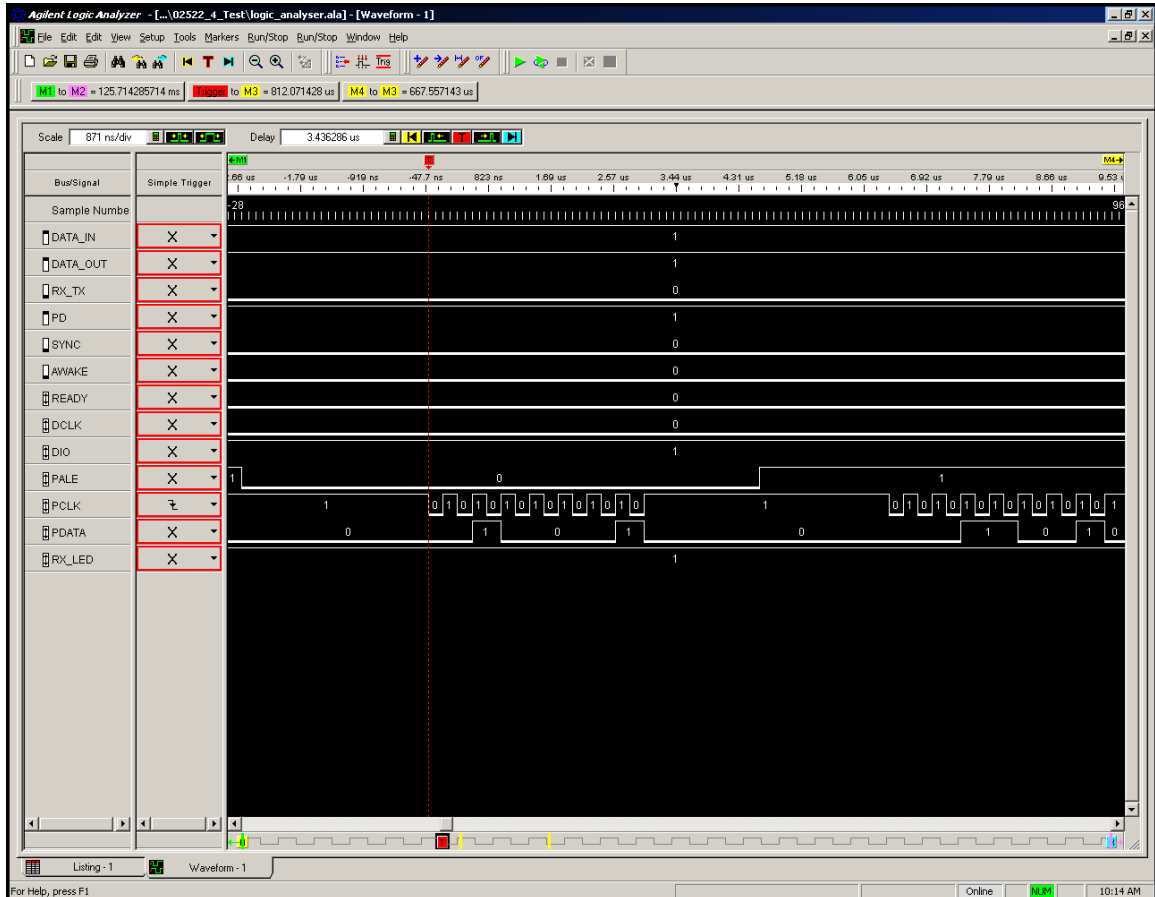
Figure 9: I/O lines during CC1000 configuration
