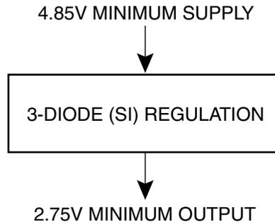
**Figure 6.** Simple Diode Regulator Circuit Diagram
