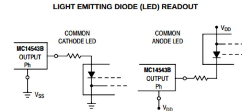
NOTE: Bipolar transistors may be added for gain (for  $V_{DD} \leq 10\text{ V}$  or  $I_{out} \geq 10\text{ mA}$ ).
