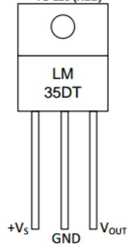
Tab is connected to the negative pin (GND).
