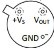
Case is connected to negative pin (GND)
