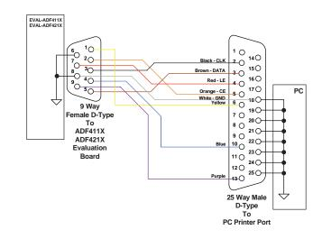
Figure 2. PC Cable Diagram
