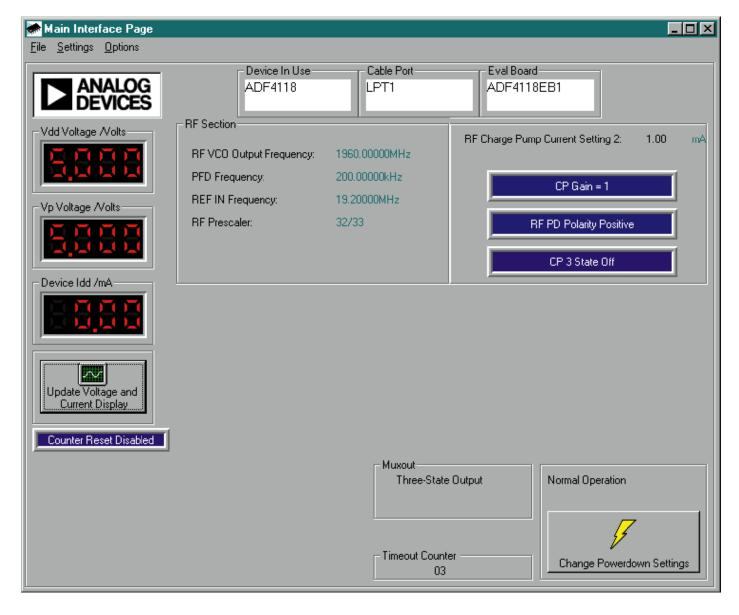
Figure 5. Software Front Panel
