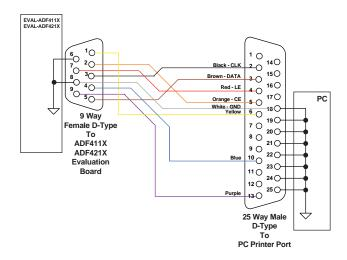
Figure 2. PC Cable Diagram
