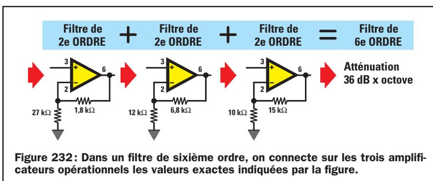
$$\begin{aligned} \text{C1 nF} &= 159\,000 : \\ &(\text{R1 kilohms} \times \text{Hz}) \\ \text{R1 kilohms} &= 159\,000 : \\ &(\text{C1 nF} \times \text{Hz}) \end{aligned}$$
