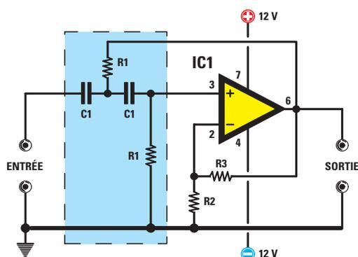
$$\begin{aligned} \text{Hz} &= \frac{159\ 000}{C1 \text{ nF} \times R1 \text{ k}\Omega} \\ C1 \text{ nF} &= \frac{159\ 000}{R1 \text{ k}\Omega \times \text{Hz}} \\ R1 \text{ k}\Omega &= \frac{159\ 000}{C1 \text{ nF} \times \text{Hz}} \\ R3 &= R2 \times 1,7 \\ R2 &= R3 : 1,7 \end{aligned}$$
