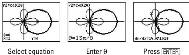
**Figure 16-17:** Steps in finding the  $dy/dx$  at a specified value of  $\theta$ .
