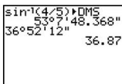
**Figure 3-5:** Converting between degrees and DMS.
