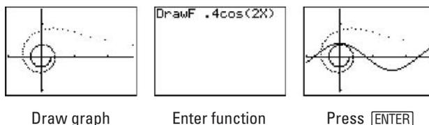
**Figure 12-3:** Steps in drawing a function on a graph.
