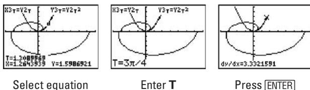
**Figure 15-12:** Steps in finding the  $dy/dx$  at a specified value of  $T$ .
