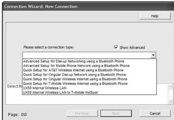
Select the *Your CLIÉ model* Internal Wireless LAN option and click Next to continue. The screen shown in Figure 15-11 appears and prompts you to enter your network's SSID. Note that some wireless networks are configured with a blank SSID; if this is the case with yours, simply leave the Network ID (SSID) field blank. Click the Next button when you're done.
