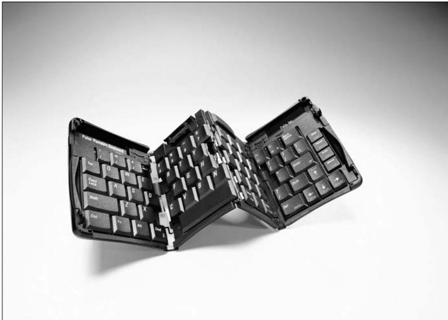
**Figure 17-3:** The original Stowaway folds into a compact package and unfolds to full laptop keyboard size.
