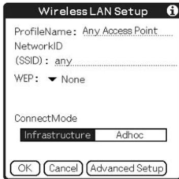
If you use WEP encryption on your home or work network, you can configure an additional profile for that access point with the proper SSID and WEP code, and select the Any Access Point profile when you're roaming outside of the home or office environment.
