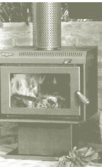
The best type of firewood heater is a slow combustion stove with an airtight firebox and an air inlet that regulates the amount of air supplied to the combustion chamber, as well as a fan to distribute the heat. They are up to 70 per cent efficient and must comply with Australian standards regarding their flue gas emissions. You can get slow combustion wood heaters in a variety of sizes, with large convection models that use a fan to distribute heat up to 130 square metres.
