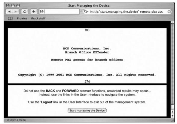
This front-end was designed to put a new face on an older PBX product, but client security seems to have been an afterthought. Notice that the interface asks the user to "Logout" of the interface, indicating that the user is already logged in. Also, notice that cryptic button labeled *Start Managing the Device*. After firing off a Google search, all a malicious hacker has to do is figure out which button to press. What an unbelievably daunting task.
