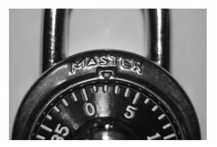
This midpoint between these digits is 1.5, which is obviously not a whole number. To find the next sticking point, release the tension on the shackle, turn the dial past the current sticking point's high boundary and reapply tension. The dial should stick again, revealing the location of the next sticking point. Some sticking points will rest on whole numbers. For example, the next photo shows that the low boundary of the next sticking point is 7.5.
