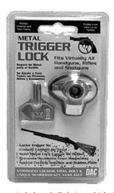
This lock consists of a typical clam shell design which shrouds the gun's trigger and guard. The halves are secured by a threaded bolt that mates to a provided key. In the locked position the head of the bolt is recessed into the lock's body. Marc and Matt discovered that a McDonald's drinking straw could be used to open the lock with relative ease, as shown in the next two photos.
