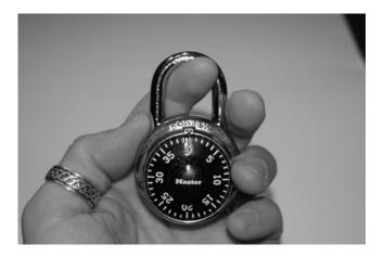
Next, begin turning the dial. If enough tension is applied, the dial should stick between two numbers. I'll call this a *sticking point*. Twelve sticking points exist on each affected lock. The first step is to find and record the location of each sticking point. For example, the lower boundary of this lock's first sticking point is, as shown in the next photo.
