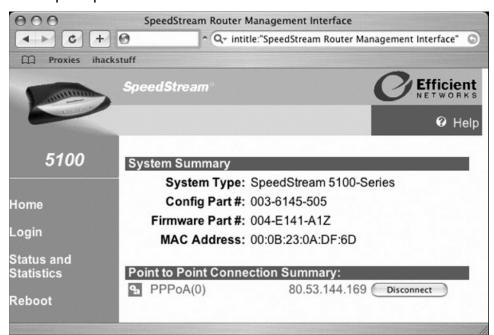
Figure 6.7 Open SpeedStream DSL Router Allows Remote Disconnects
