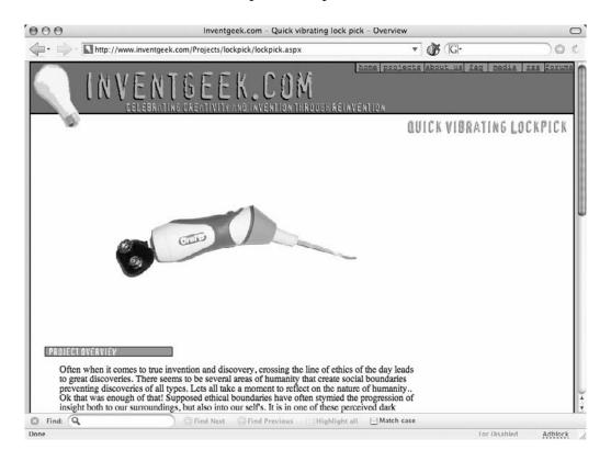
This hack involves modifying the flosser to accept a stronger power source. Then the flosser, when inserted into a lock, can vibrate hard enough to jiggle tumblers out of the locked position. Be sure to check out www.inventgeek.com for more information, and be sure to full-body tackle anyone you see skulking around with an electric flosser. They're definitely up to something.
