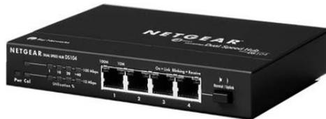
Figure 1-3: A typical four-port Ethernet hub
