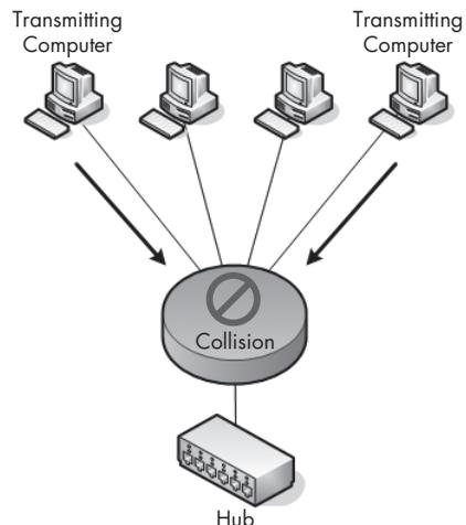
Figure 2-3: Collisions occur on a hub network when two devices transmit at the same time.
