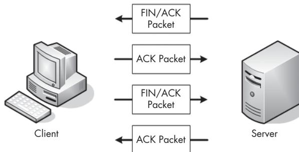
Figure 6-9: The FIN/ACK handshake process gracefully terminates a TCP connection.
