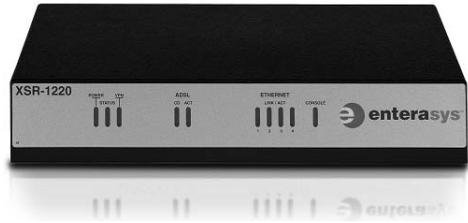
Figure 1-7: A small router suited for use in a small network
