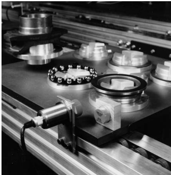
Figure 13.60 Individual components of a clutch release stop on a revolving pallet. Transponder and reader antenna are visible in the lower part of the photo (reproduced by permission of Pepperl & Fuchs GmbH, Mannheim)
