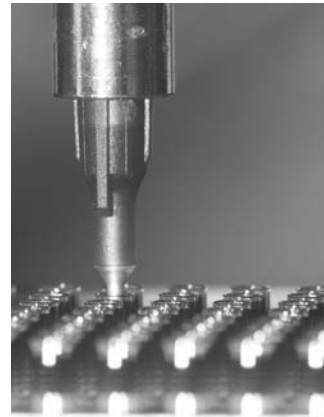
Figure 12.3 Left: aligning glass tube sections on the workpiece carrier. Right: dosing epoxy resin for a later bonding of ferrite and chip (reproduced by permission of AEG Identifikationssystem GmbH, RFID im Blick)
