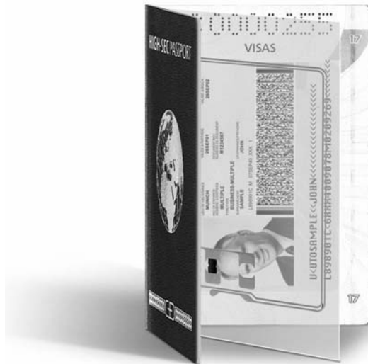
Figure 13.18 Position and design of the RFID antenna in ePassports. The microprocessor chip can be recognized as a small black point over the passport photograph. (reproduced by permission of Giesecke & Devrient GmbH, Munich)
