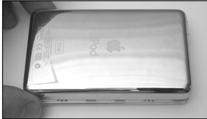
Figure 11.35 Snapping the Case Back Together
