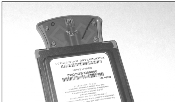
Figure 10.7 Inside the Antenna Compartment
