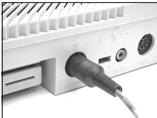
Figure 8.70 We're Done! The Final Atari 8-Bit S-Video and Composite Cable
