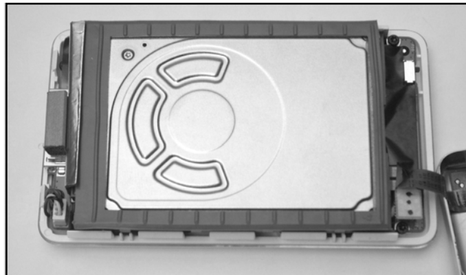
Figure 11.34 Hard Drive Back in Place
