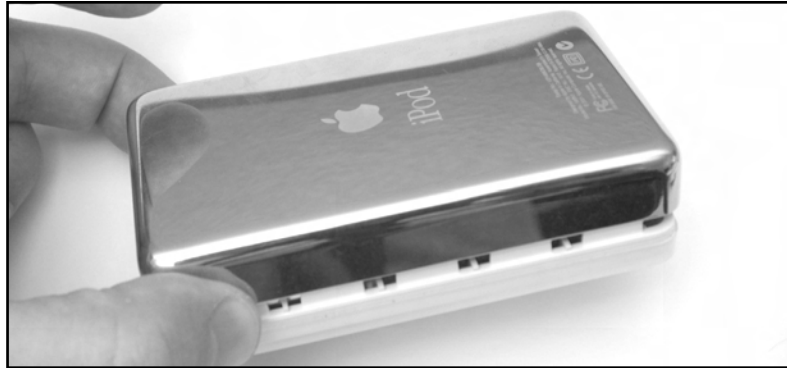
Figure 11.23 Reattaching the Metal Half of the Case
