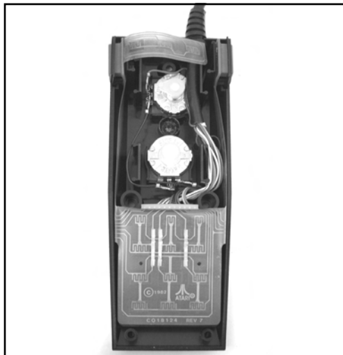
Figure 8.22 Bottom Half of 5200 Controller
