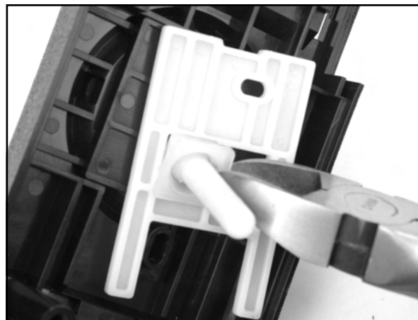
Figure 8.26 Freeing the Joystick
