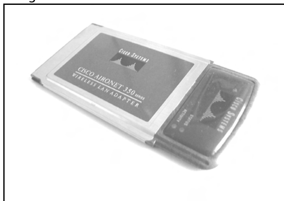
Figure 10.1 A Cisco Card with an Integrated Antenna
