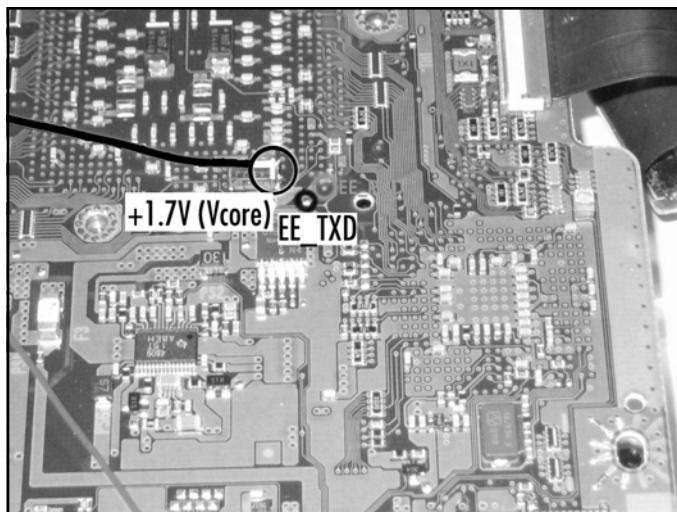
Figure 9.11 The V CORE , EE_TXD, and EE_RXD
