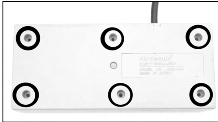
Figure 7.11 Bottom of NES Control Pad
