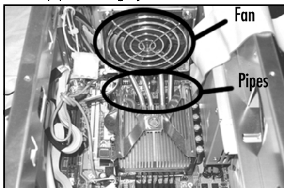
Figure 6.28 The Shuttle Heatpipe Cooling System
