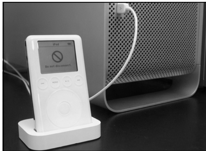
Figure 11.36 Charging the new Battery
