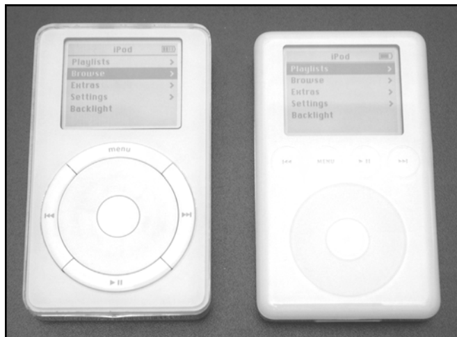
Figure 11.1 The 5GB First-Generation iPod (Left) and the 20GB Third-Generation iPod (Right)
