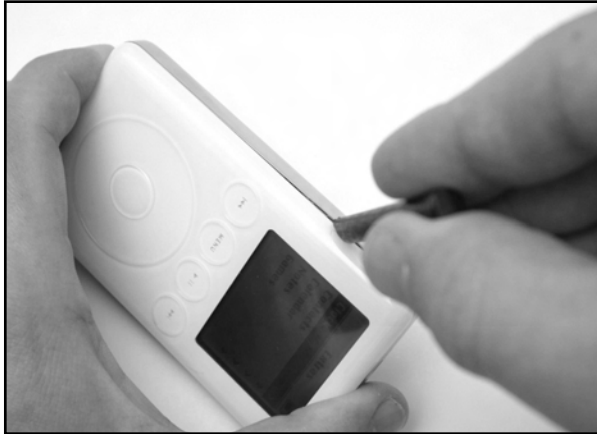
Figure 11.10 Prying into the Case
