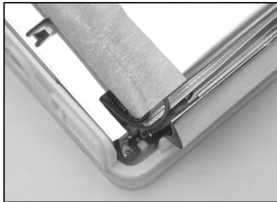
Figure 11.22 Power Cable Safely Tucked Away
