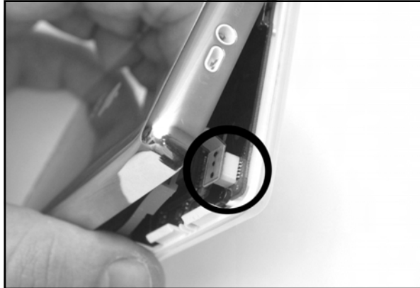
Figure 11.14 Connector Holding Two Halves Together
