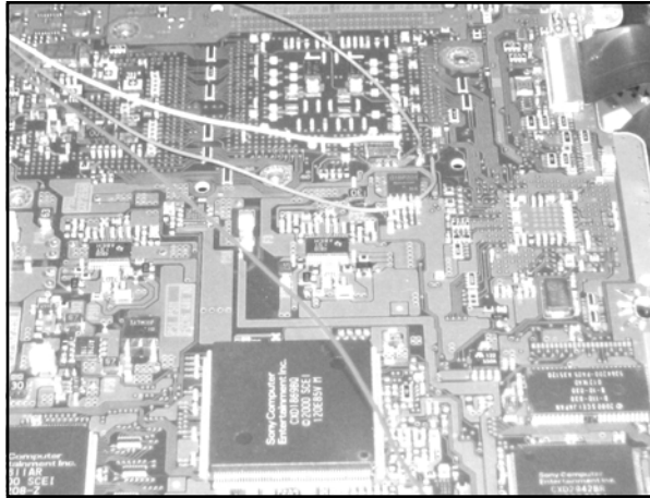
Figure 9.12 Installed SIO Wiring
