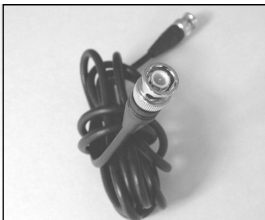
Figure 10.4 An Unmodified Thinnet Cable
