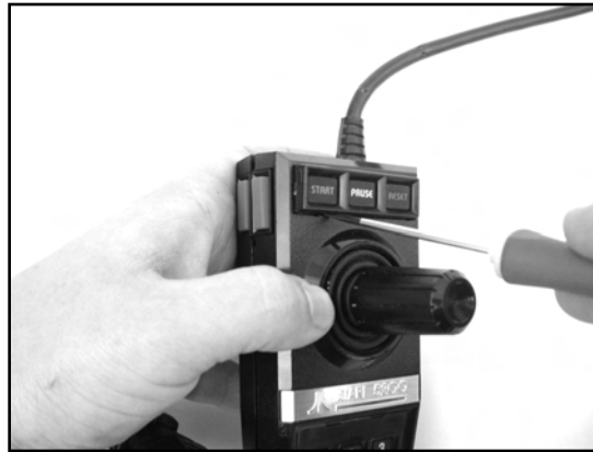
Figure 8.21 Removing the Upper Bezel
