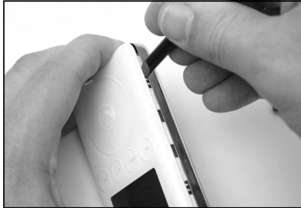
Figure 11.12 Unclip all the Tabs
