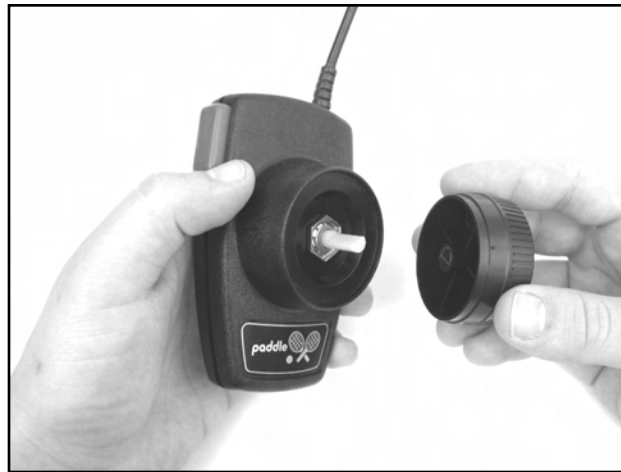
Figure 8.16 Removing the Paddle Dial
