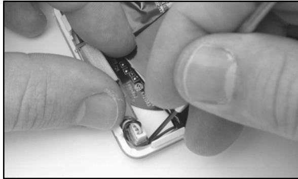
Figure 11.31 Tucking In the Power Cable
