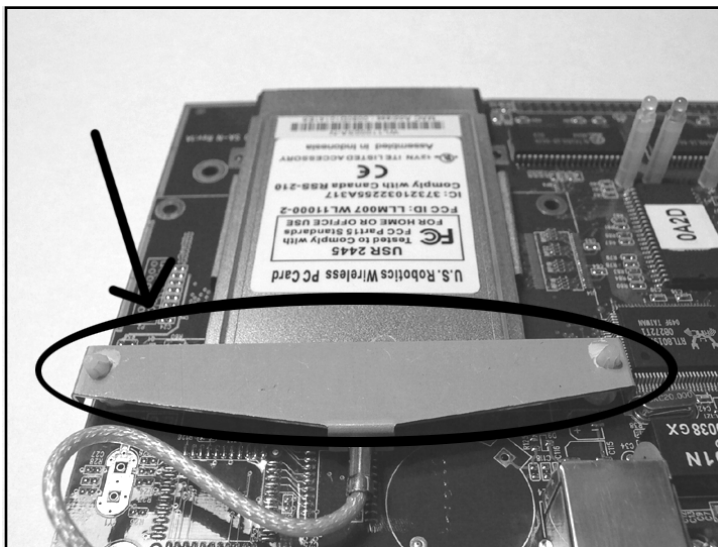
Figure 10.15 Before Removing the Card ... See the Metal Brace?
