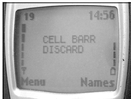
Figure 12.31 Test 19: Ignoring Barred Base Stations
