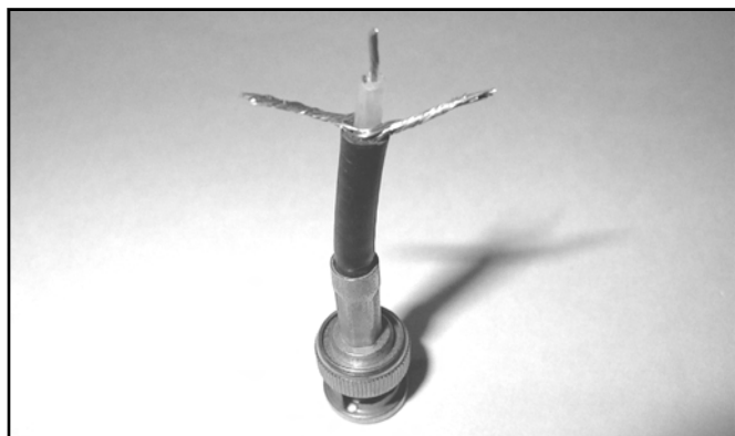
Figure 10.10 A Prepared BNC Connector Ready for the Hack
