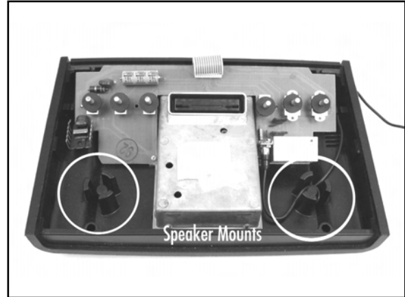
Figure 7.23 Receptacles Inside the Case for Speakers
