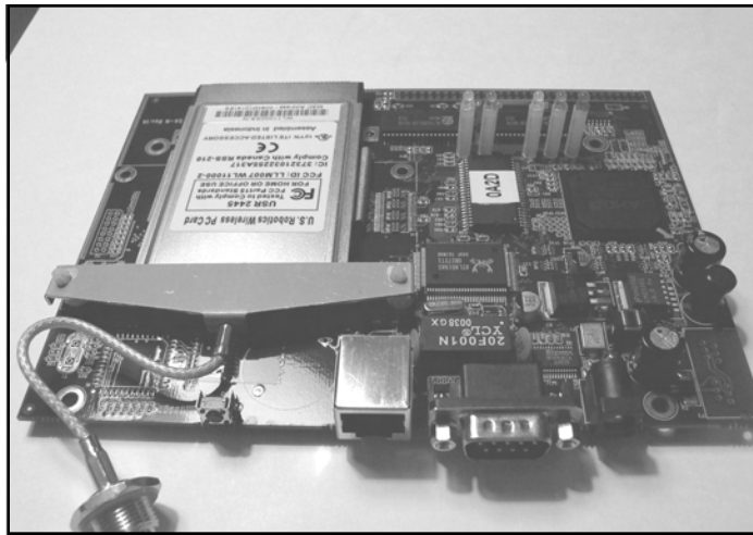
Figure 10.14 The AP with the Cover Removed
