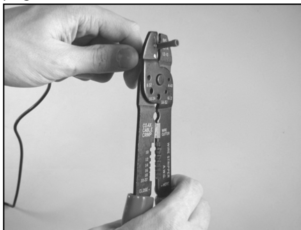
Figure 5.47 Crimping the Wire
