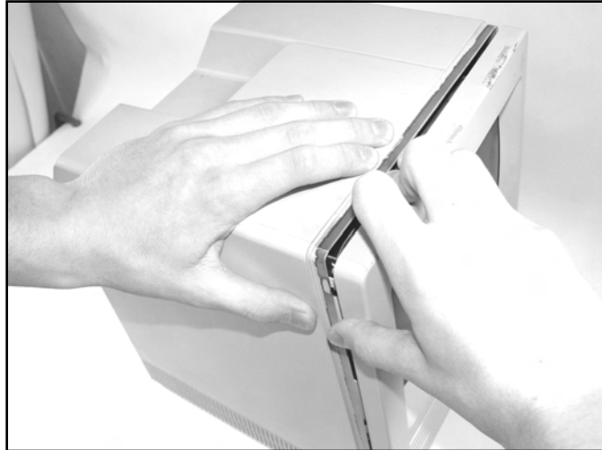
Figure 5.4 Prying the Case Apart
