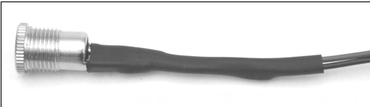
Figure 8.44 Building the Power Cable
