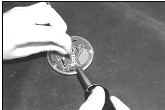
Figure 5.63 Soldering the LED
