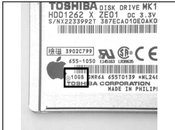
Figure 11.38 Drive Capacity Printed on the Hard Drive Sticker
