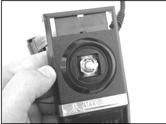
Figure 8.29 Assembling the 2600 Potentiometer
