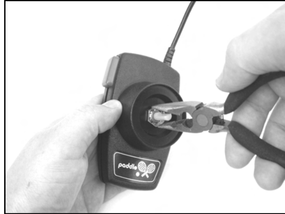
Figure 8.17 Removing the Paddle Nut
