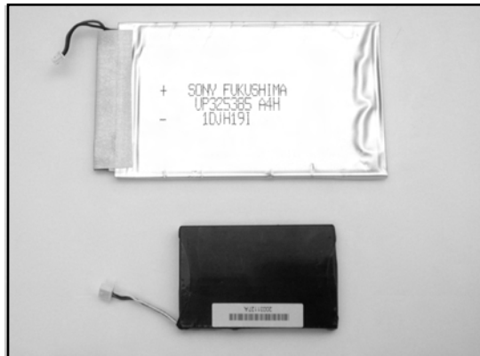
Figure 11.15 iPod Batteries: First- and Second-Generation (Top) and Third-Generation (Bottom)
