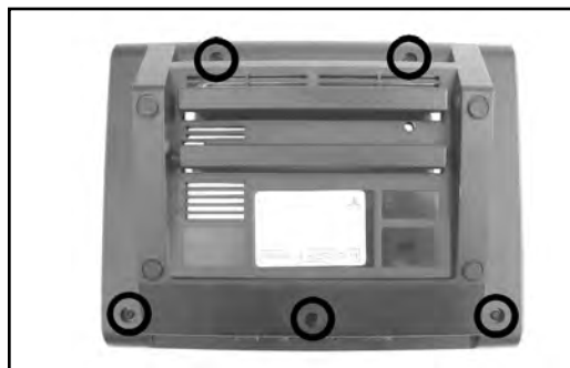
Figure 7.37 Remove Screws as Shown
