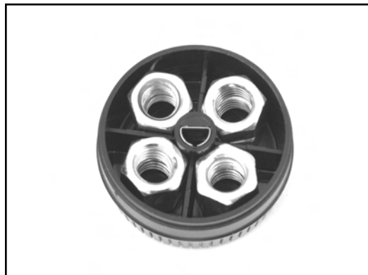
Figure 8.33 Weighing Down the Dial with Hex Nuts
