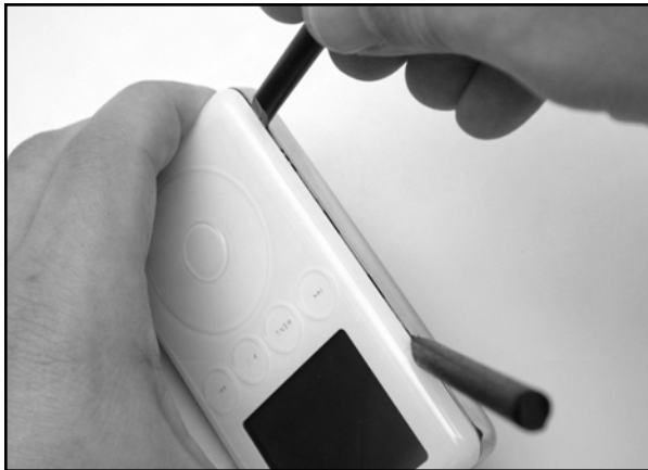
Figure 11.11 Continue Prying Along One Side
