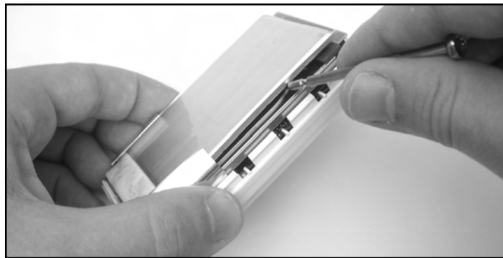
Figure 11.40 Pulling the Battery and Hard Drive Apart
