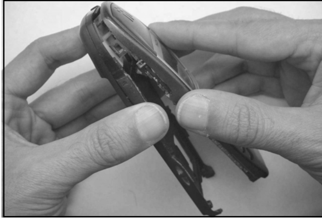
Figure 12.7 Releasing the Top Clips
