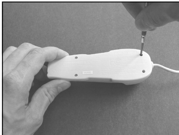
Figure 3.4 Unscrewing the CueCat
