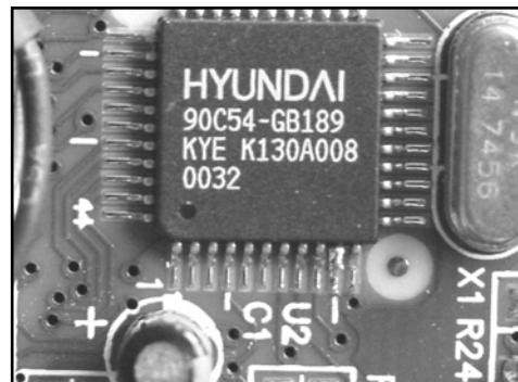
Figure 3.34 Hack Complete: Pin 10 of Microprocessor Lifted (Close-Up)
