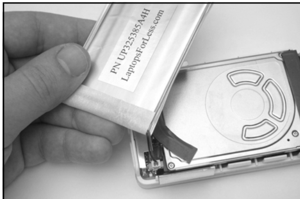
Figure 11.20 Connecting the New Battery
