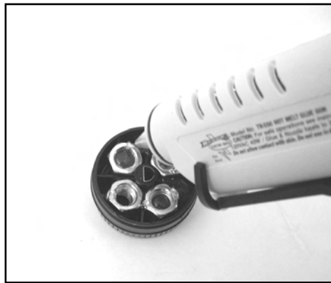
Figure 8.34 Gluing the Nuts in Place
