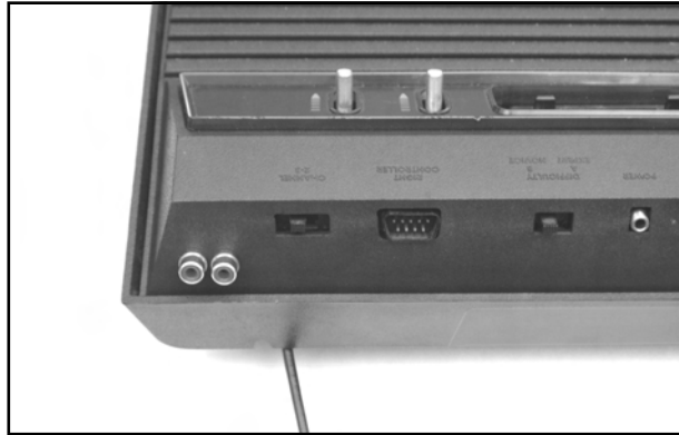
Figure 7.35 Stereo Jacks on Outside of Case
