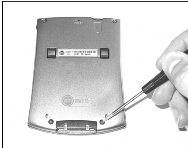
Figure 13.29 Unscrewing the Palm m505
