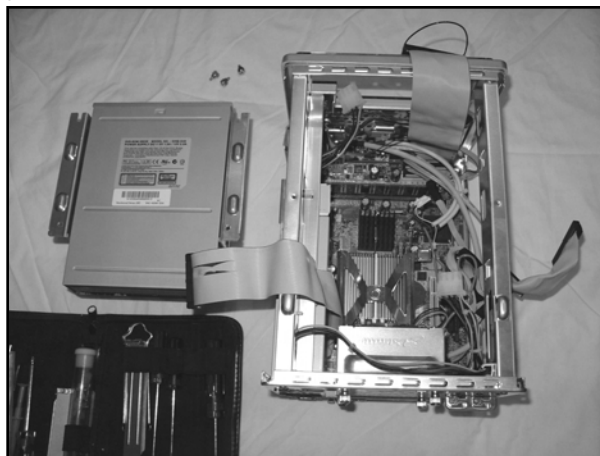
Figure 6.27 Removing Parts from the Shuttle Case
