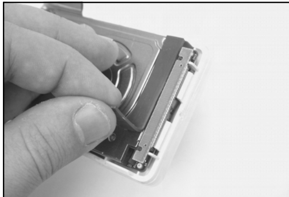
Figure 11.42 Removing the Rubber Pads
