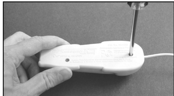
Figure 3.9 Unscrewing the CueCat
