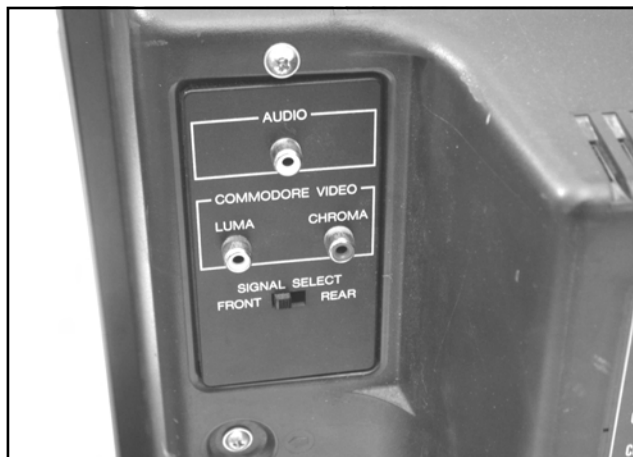
Figure 8.71 Commodore 1702 Rear Input Jacks
