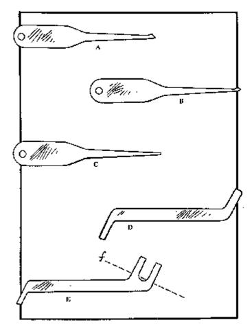
Figure 3. A; a diamond pick; B: a small diamond pick; C: a tubular cylinder lock pick; D: a tension wrench, used with the diamond picks; E: a tension wrench intended for double-wafer cylinder locks and tubular cylinder locks.
