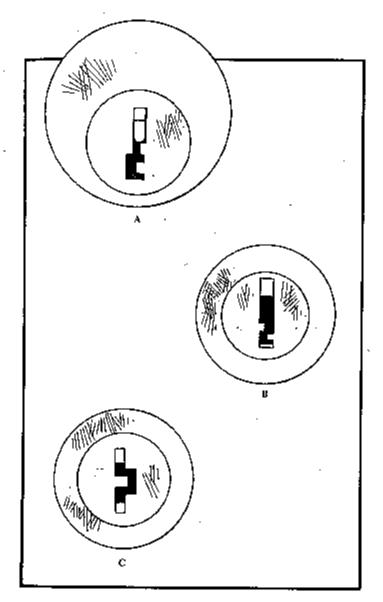
Figure 6. A: a pin tumbler lock; B: a wafer tumbler lock; C: a doublewafer tumbler lock.
