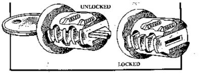
Figure 13. A wafer tumbler lock.
