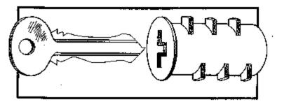
Figure 16. A double-wafer lock.
